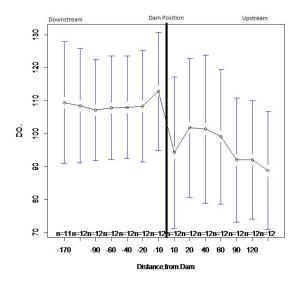
Figure 2A. Mean plot of Dissolved oxygen levels upstream and downstream of impoundment
