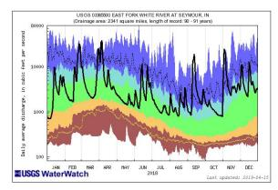
Figure 9. Hydrograph of East Fork of the White River during 2018. During study duration (June) flood events are observable.
