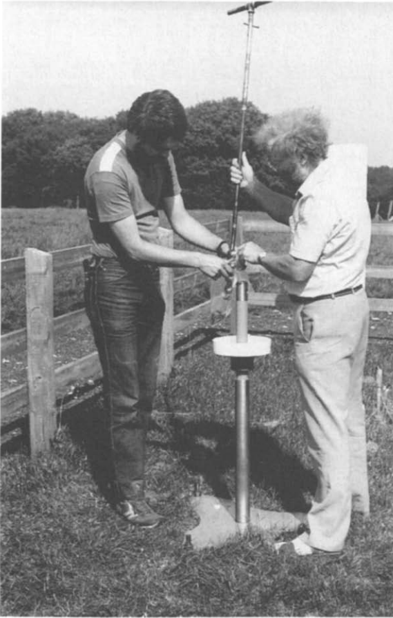
Fig. 5. An access tube being installed; a calibration sample is being transferred from auger to plastic bag for gravimetric determination of moisture.
