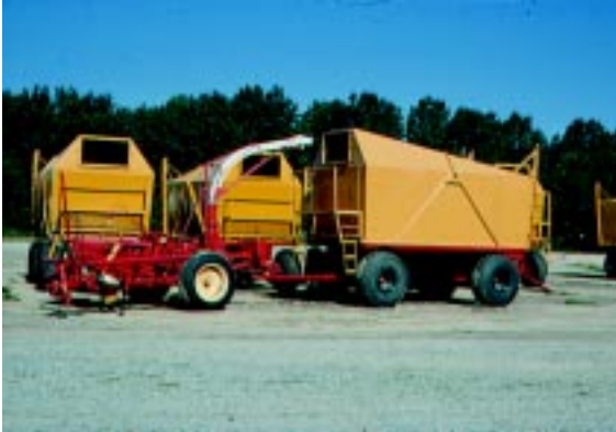
Mint distillation tubs are generally custom-built by the grower. Tubs are about 6 inches wider at the top than at the bottom. This shape helps to pack down the chopped mint as it is blown into the tub.
