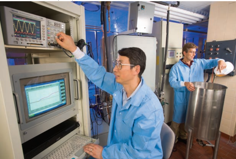
In studies of methods to pasteurize liquid foods such as apple cider without using heat, research leader Howard Zhang (left) and chemical engineer David Geveke develop and evaluate pulsed electric field and radio frequency electric field treatments.
