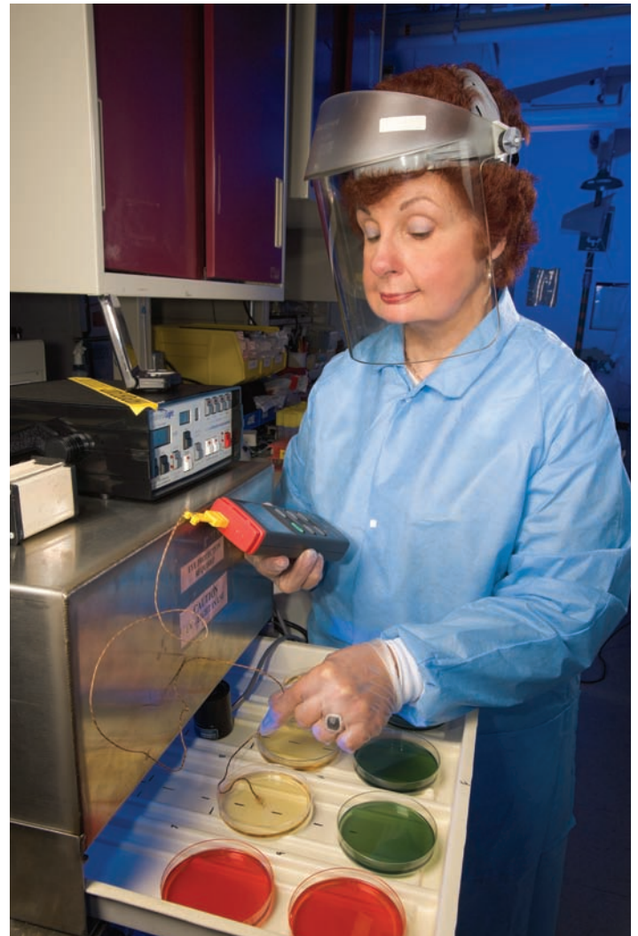
Food microbiologist Kathleen Rajkowski evaluates how well a pulsed ultraviolet light treatment inactivates bacterial pathogens on the surface of test media.
