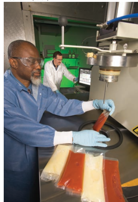
Food microbiologist Dike Ukuku (left) and engineer Joseph Sites evaluate effects of high-pressure processing on microbial stability of tomato juice and liquid eggs.
