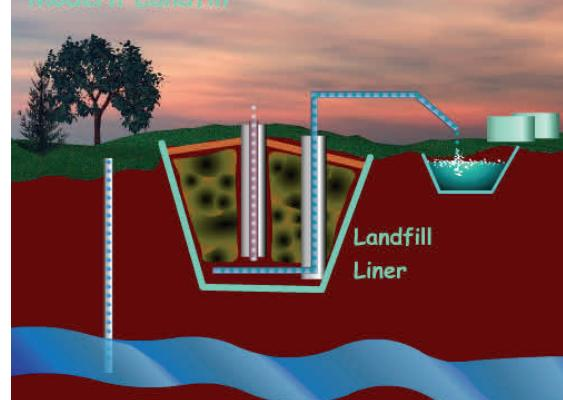
A landfill has clay and plastic liners to keep the pollutants from reaching the water table. A series of leachate tubes at the bottom of the landfill carry the contaminated water to the treatment plant.
