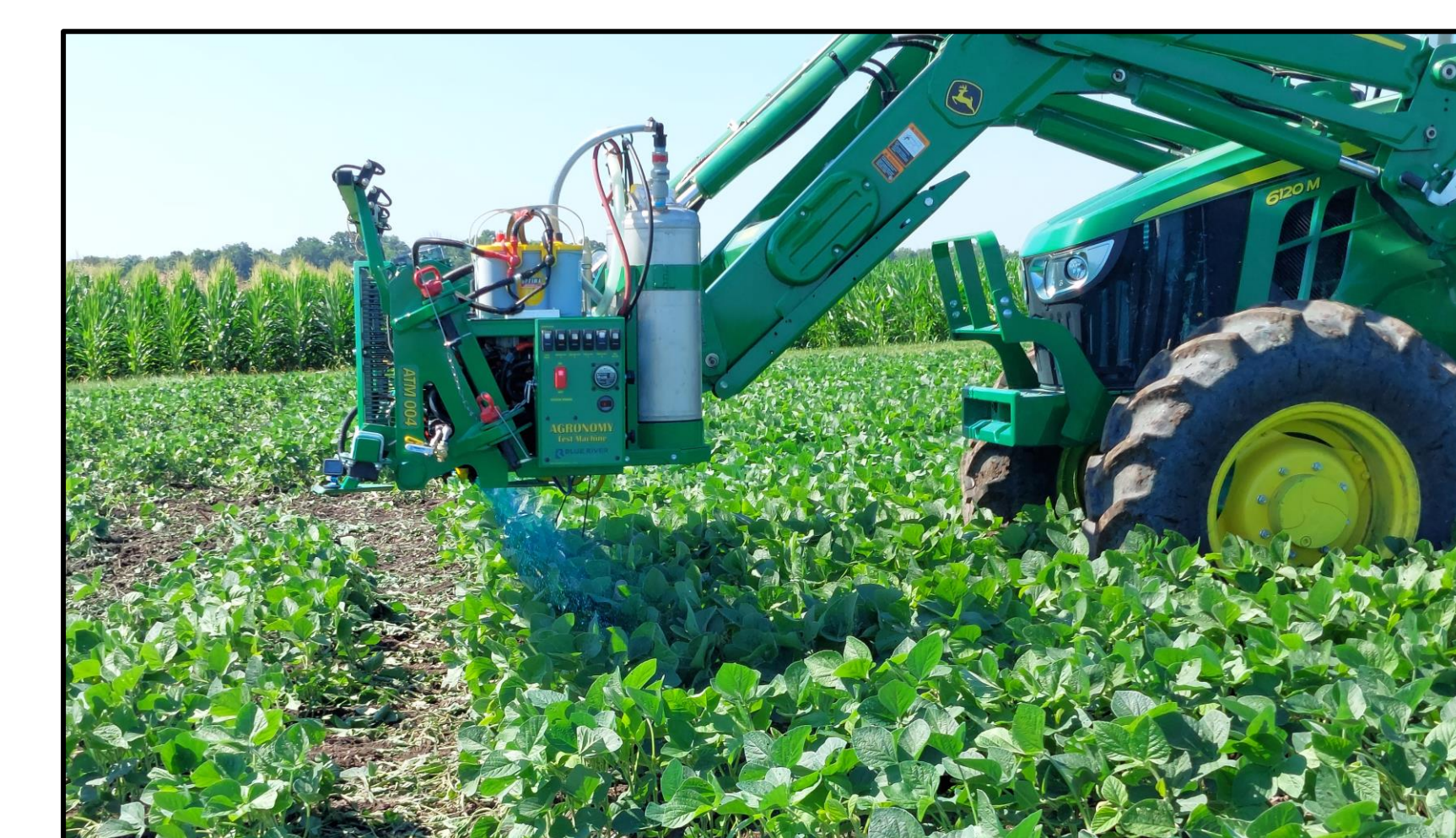
Figure 4: Blue River Technology Agronomic Testing Machine equipped with a dual tank delivery for site-specific applications.
