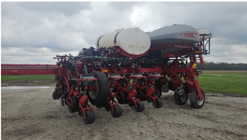
Figure 1a. A 12-row Case 2150 planter with vacuum meters, active hydraulic downforce, and row cleaners.
