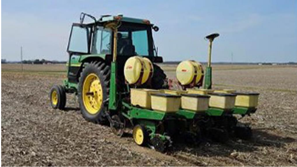
Figure 1b. A 4-row John Deere 7200 planter with finger-pickup meters, spring downforce, and no row cleaners.
