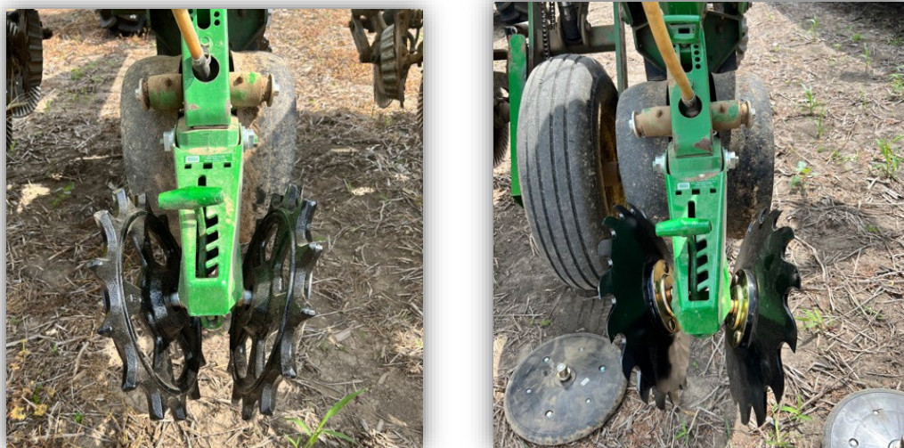
Figure 4. Photos of the two aftermarket closing wheels which were tested in comparison to the standard rubber closing wheel. Cruiser Extreme from Copperhead Ag (Left) and the Cupped Razor from Martin-Till (Right). Both closing wheels are marketed for high-residue systems and were set to manufacturer specifications.
