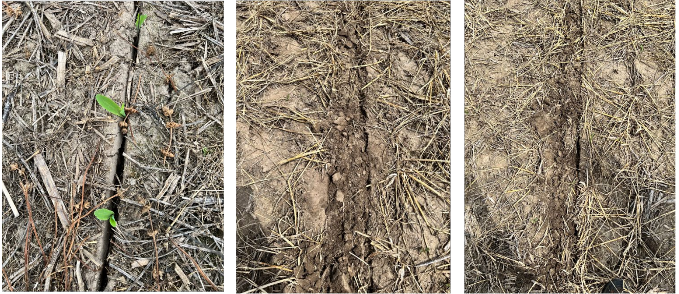
Figure 5. Observed differences in furrow closure and seed-to-soil contact between the standard rubber closing wheel (Left, 6 DAP), the cruiser extreme closing wheel (Middle, 1 DAP), and the cupped razor closing wheel (Right, 1 DAP).
