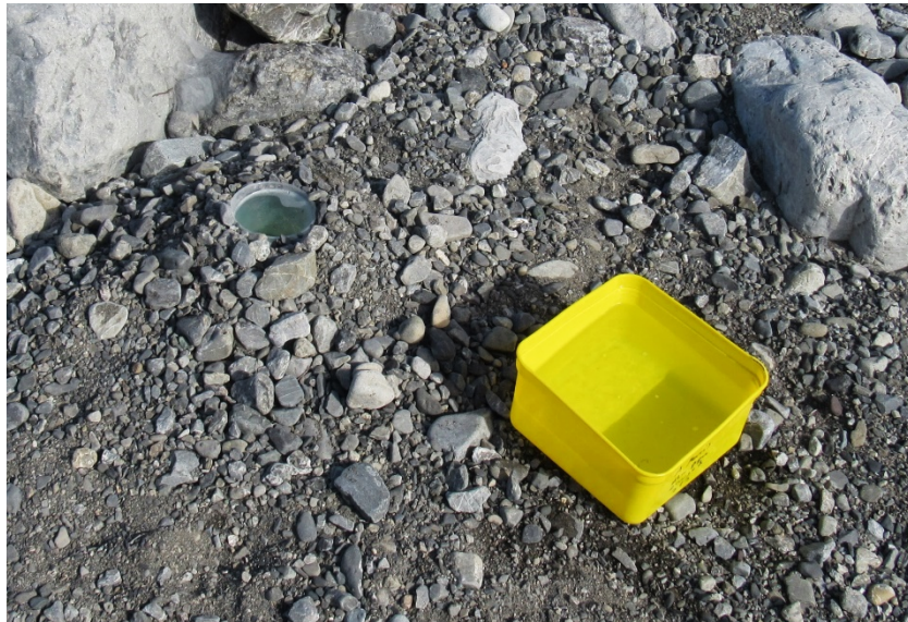
Figure 4: A pitfall trap (left) and yellow pan trap (right) are set in a river habitat plot.
