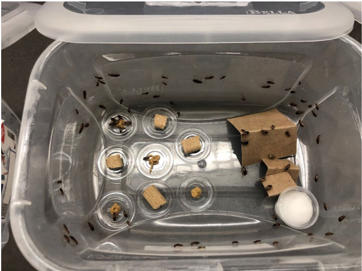
Figure 1. Interior view of a nymph bioassay arena with 4 placements of gel bait and rodent diet along with cardboard harborage and a water source.
