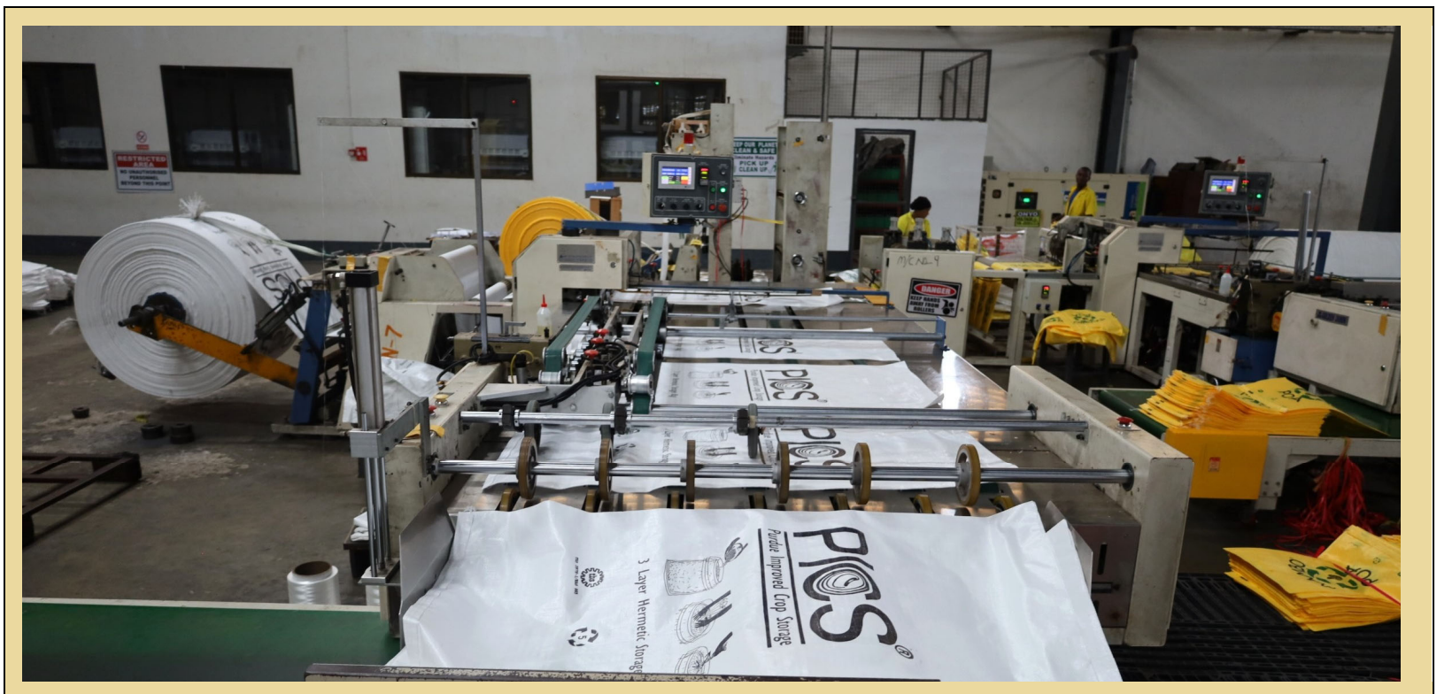
Rolls of PICS liners being cut and sealed in the P.P.T.L. factory, Tanga, Tanzania
