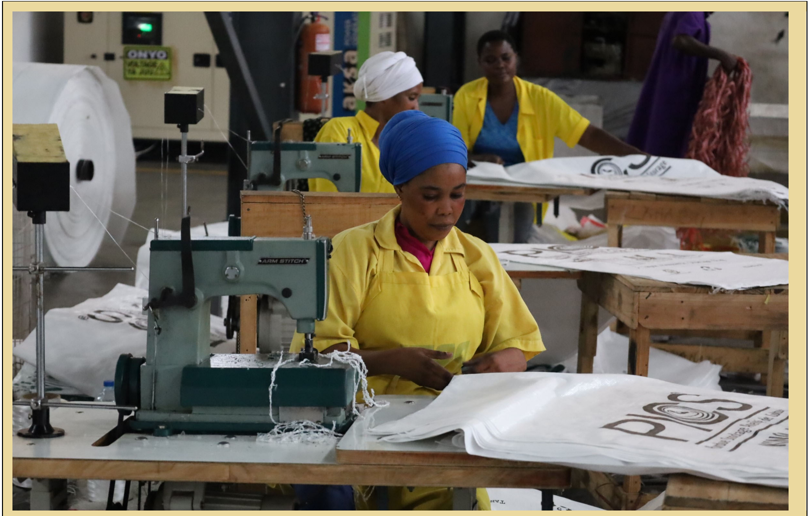
Women sewing the bottom and stitching the top of PICS woven bags in the P.P.T.L. factory, Tanga, Tanzania.
