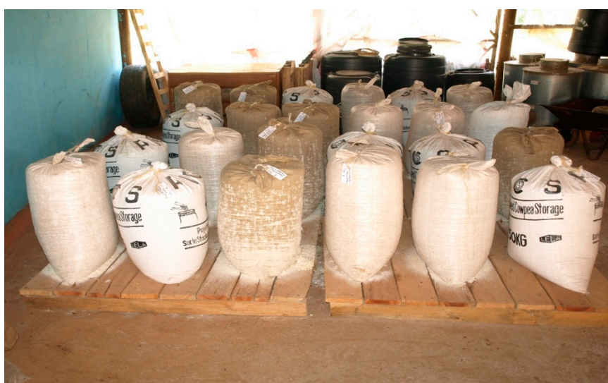
Figure 2. Side by side storage of PICS, PP and Jutes bags during the experiment at the KARLO research station in Kiboko, Kenya. Insects seriously damaged PP and Jute treatments, as reflected in the dust produced.
