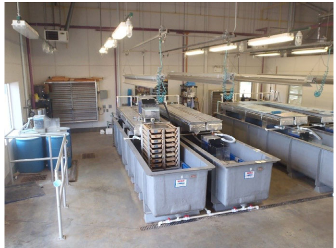
FIGURE 1. Recirculating aquaculture systems for Eastern hellbender propagation at Shepherd of the Hills State Fish Hatchery (SHFH). The large gray tanks serve as support structures for the insulated aluminum hellbender rearing tanks with their lids, filtration units, and blue sumps. This area of flow-through fish production has been converted into the RAS for hellbender production.
