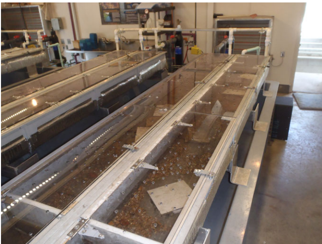
FIGURE 3. Linear tanks fitted with Lexan lids for biosecurity. There are three sections per tank, each having a hinged and hasped area for a padlock.
