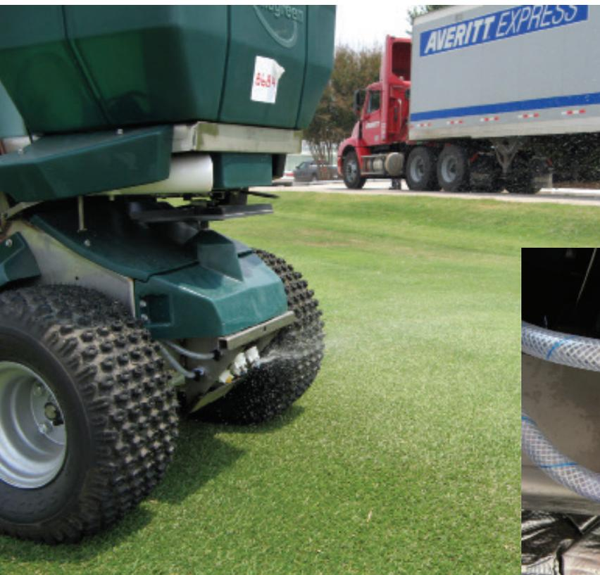
Most single-nozzle (boomless) sprayers actually have a cluster of nozzles under the front center of the sprayer. Although there are multiple nozzles, you should only use one at any time. The ability to select nozzles permits quick and accurate changes in spray width for trim and broadcasting or when changing ground speed. You must calibrate each nozzle and speed combination on the sprayer.
