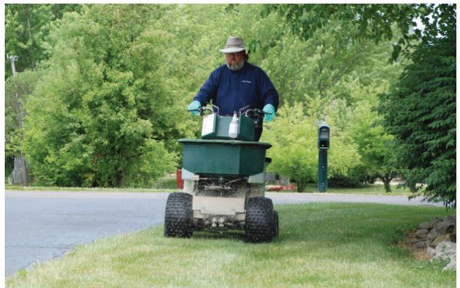
**The edge guard (deflector) is a physical barrier that prevents the fertilizer from going onto impervious surfaces. Without a guard, the spreader shown below would apply fertilizer onto the paved surface. Always blow or sweep fertilizer off any sidewalks back into the turf.**
