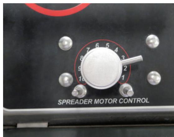
**Some units may have a hydraulic impeller motor that can adjust the spread width. When you calibrate one of these units, note the setting you are using. If you adjust this setting you will need to recalibrate.**
