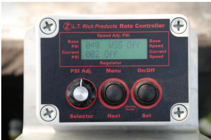
A rate controller can help you maintain a constant application rate despite changes in travel speed.
