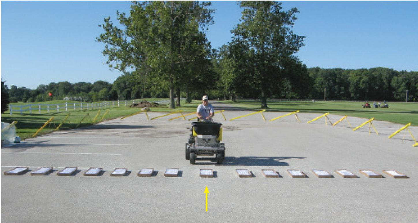
The center box is marked with an arrow. Notice the extra space on either side of the center box to allow room for the wheels. In this example, the spreader is being calibrated for a product with a large granule, so the boxes are placed about 12 inches apart to catch the granules along the entire width of the spread.
