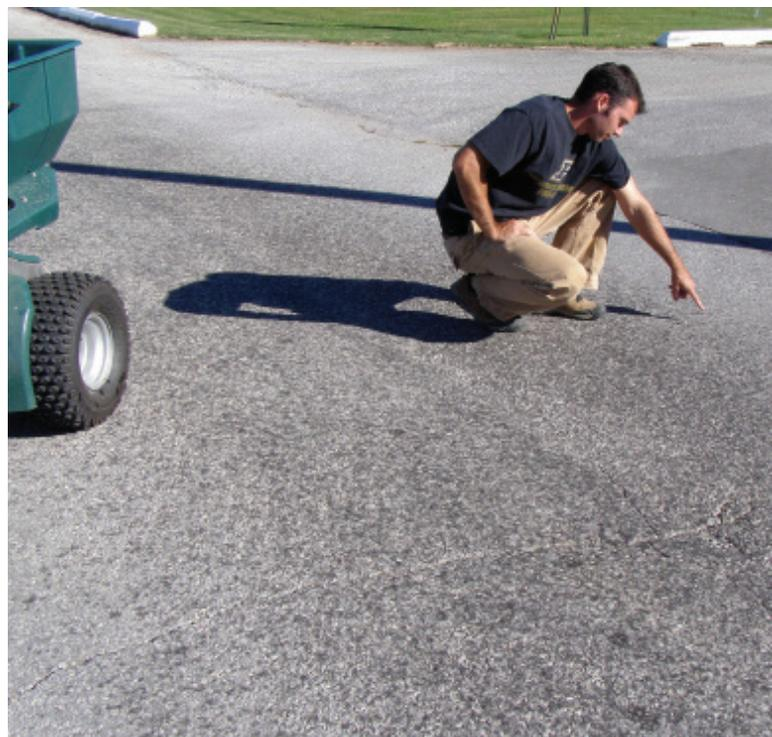
**Locate each edge of the spray pattern where the pavement is consistently wet. Measure from edge to edge to get the effective spray width.**
