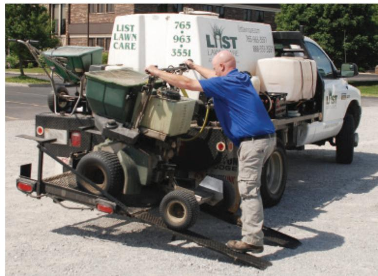
This carrier was specially built to haul ride-on sprayers. Some carriers feature passive restraint systems that improve safety and ease of unloading and loading. These carriers don't require trailers, which means operators can haul ride-on equipment with compact vehicles that are easier to maneuver in residential neighborhoods. Typically, a vehicle needs a heavy-duty hitch to carry these units.
