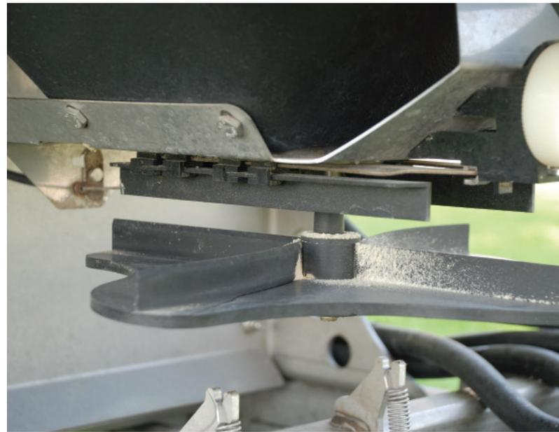
**A rotary spreader's distribution pattern can change when granular dust builds up on the spinner (impeller). Clean the spinner on a regular basis to keep the application accurate.**
