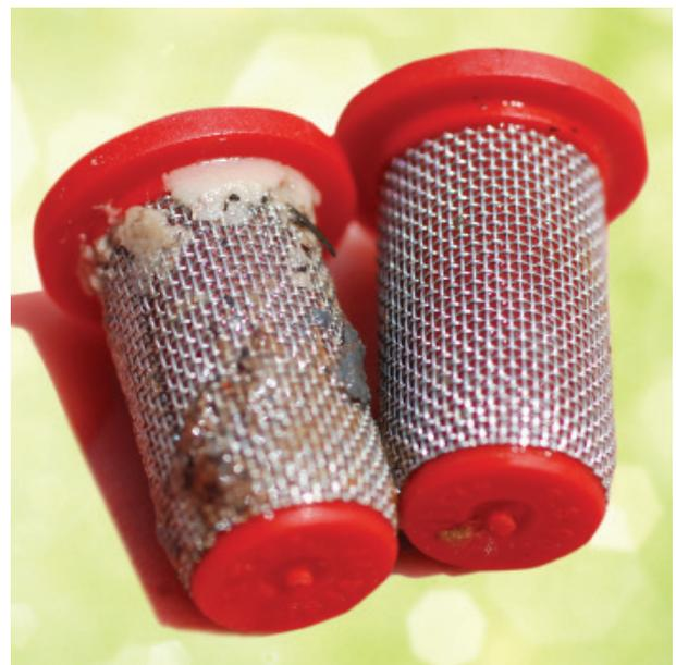
**Something as simple as a partially clogged screen (left) can undermine any calibration by altering the flow of water. Clean screens (right) can help keep sprayer output consistent. Remember to clean any filters between the spray tanks and nozzles.**
