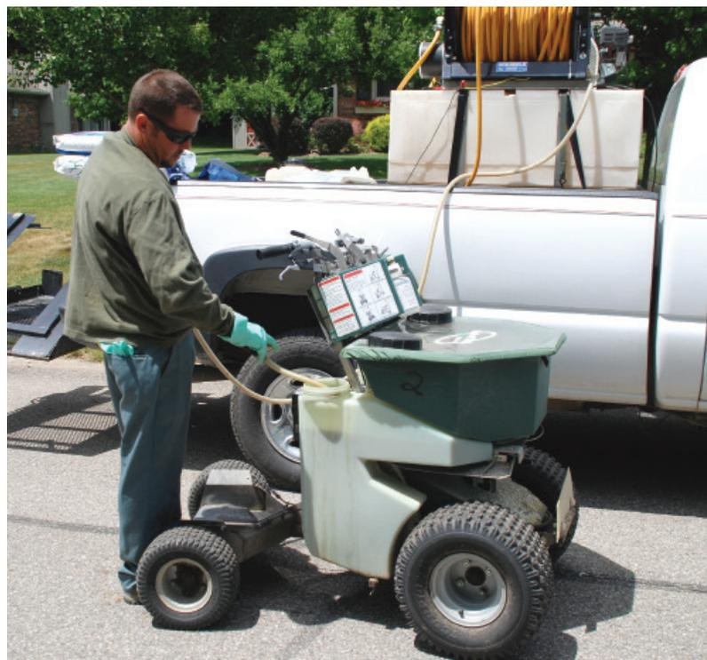
**Ride-on sprayers have relatively small tanks, so many lawn care companies use large storage/supply tanks in their trucks to refill sprayers. To be effective, the products in such tanks must be mixed for use in ride-on equipment.**
