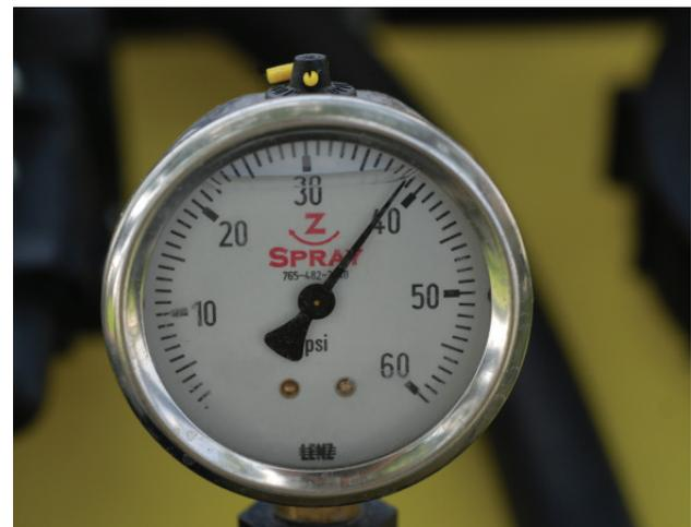
Record the nozzle pressure used during the initial calibration steps. Although changing speed or nozzle size is the best way to adjust your calibration volume, you can also modify nozzle pressure on some models to make small adjustments to output.
