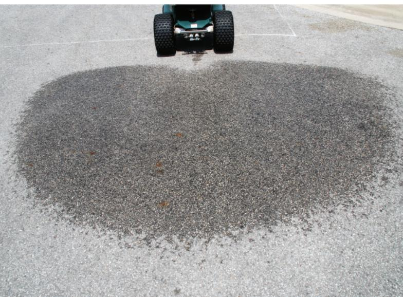
**Check the nozzle distribution pattern while the sprayer is parked and spraying at the same RPM and pressure as during the calibration run. This nozzle has a uniform spray pattern.**
