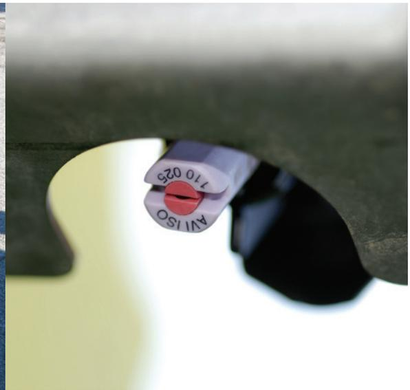
A boom-type ride-on sprayer (left) and one of the nozzles along its boom (right).
