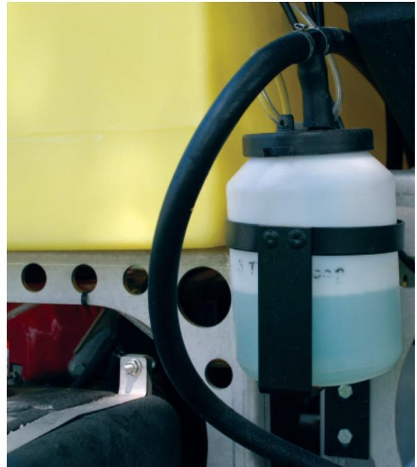
**A foam marking system comes with a tank to fill with foamer to mark the edges of your spray pattern.**
