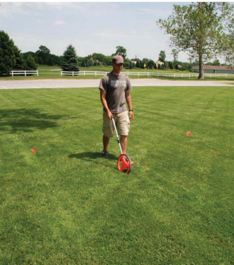
**Use a measuring tape or wheel to measure the length of a calibration course.**
