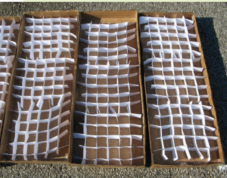
These custom 1-foot by 3-foot collection boxes were made from cardboard scraps and packing tape.
