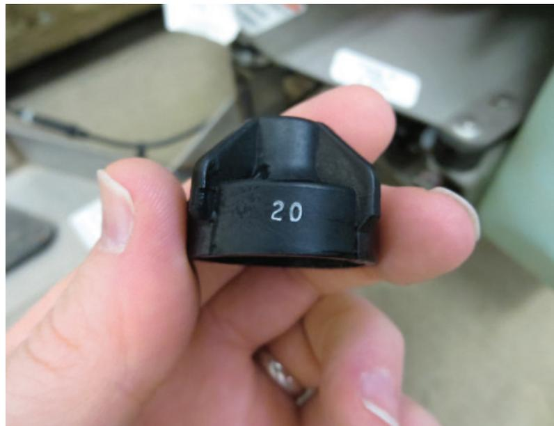
**You can adjust the pressure from 20 to 30 psi on the diaphragm-type antidrip valve on Permagreen® models. This slightly increases the effective spray width.**
