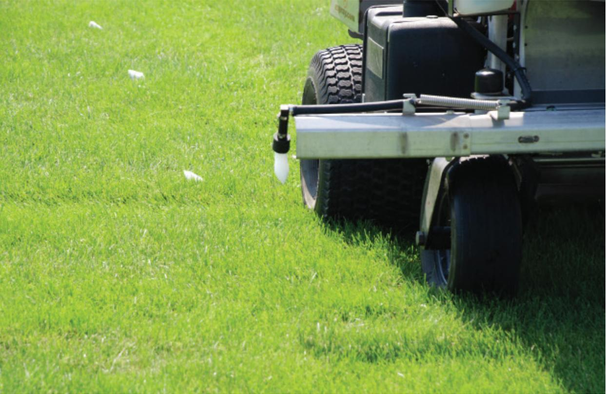
**This boom sprayer has a foam marking system that marks the edges of the spray pattern.**
