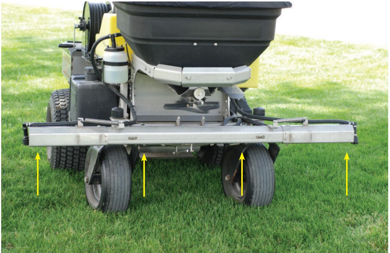
A boom-type ride-on sprayer/spreader with four nozzles. Arrows point to nozzle placement.
