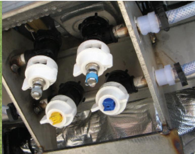
This single-nozzle boomless ride-on sprayer has four nozzles, but it only uses one at a time.
