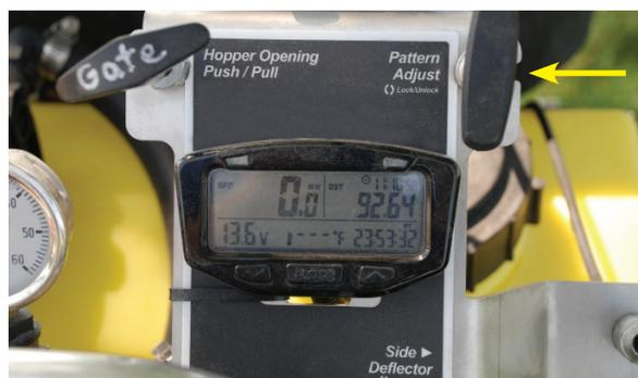
The pattern adjustment lever varies by spreader model. You control the pattern on a PermaGreen® with the third hole adjustment operating lever (top). You control the Z-Spray Intermediate® (bottom) with a pull knob.
