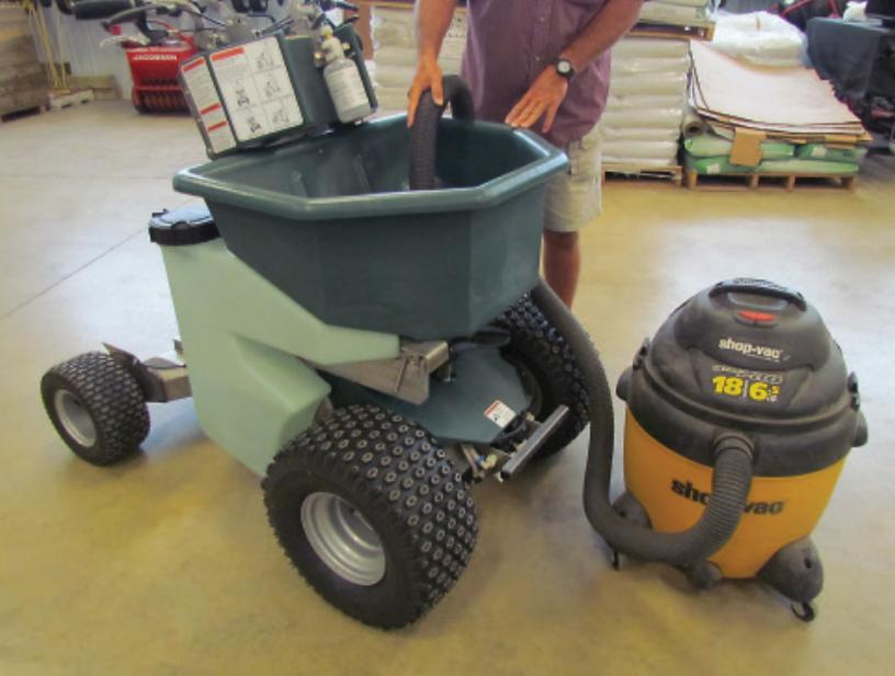
A shop vacuum will help you remove the fertilizer that was left in the hopper. Subtract what's left from the amount you started with to calculate how much fertilizer you applied to the calibration course.
