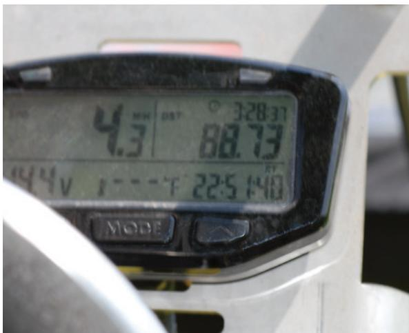
If your sprayer has a speedometer, record the speed that was used during the calibration.
