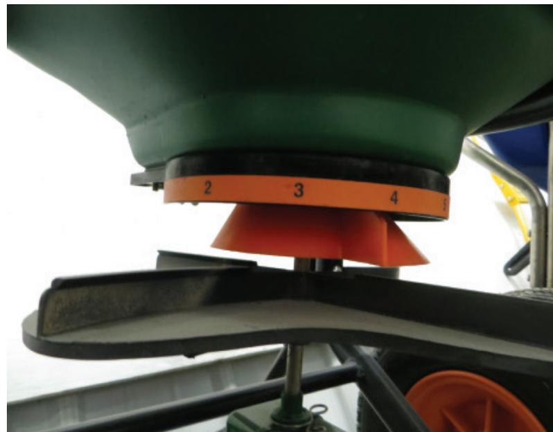
This spreader uses a rotating conical distribution device to adjust where the fertilizer hits the impeller, which adjusts the spread pattern.
