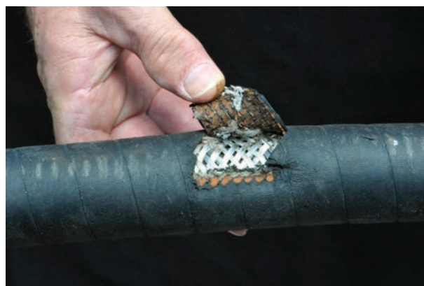
(Top) This cross-section of a new hose shows that it has an inner core surrounded by rubber and reinforcement strands. (Bottom) Cutting away a layer of the hose reveals reinforced materials.
