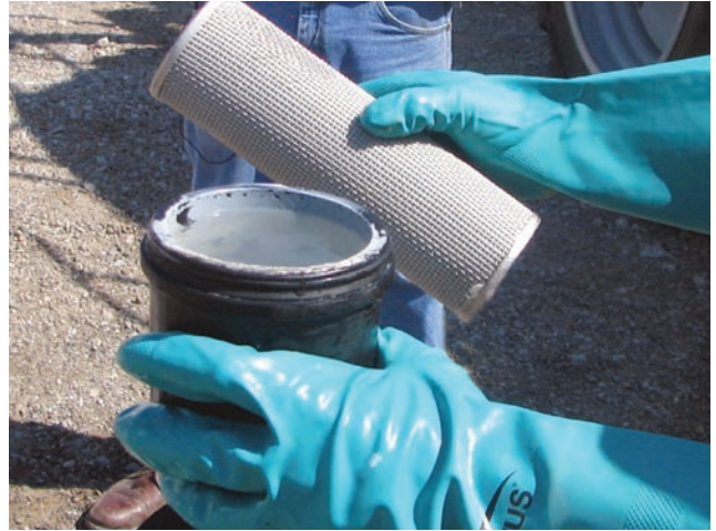
Remove the strainer and empty any water inside.
