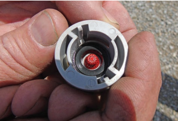
Remove nozzle bodies from the sprayer to protect O-rings. Always use gloves.
