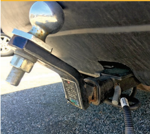
This receiver is rusted.
