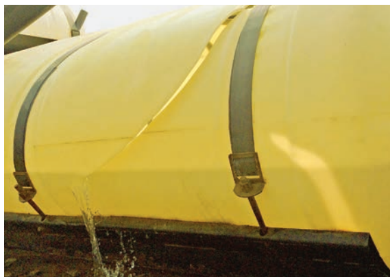
(Left) The walls of this spray tank show initial signs of ultraviolet radiation damage. (Right) This tank shows advanced stages of ultraviolet damage — note how the plastic is breaking down.
