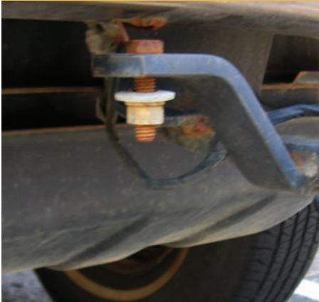
This bolt is no longer attached.
