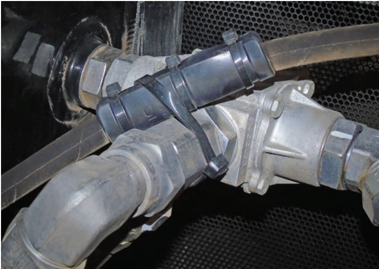
(Top left and right) These hoses have a protective sleeve. (Bottom left) The operator has wrapped a suction hose around a pressure hose to act as a protective cover. (Bottom right) This operator created a barrier between the hose and the metal frame.
