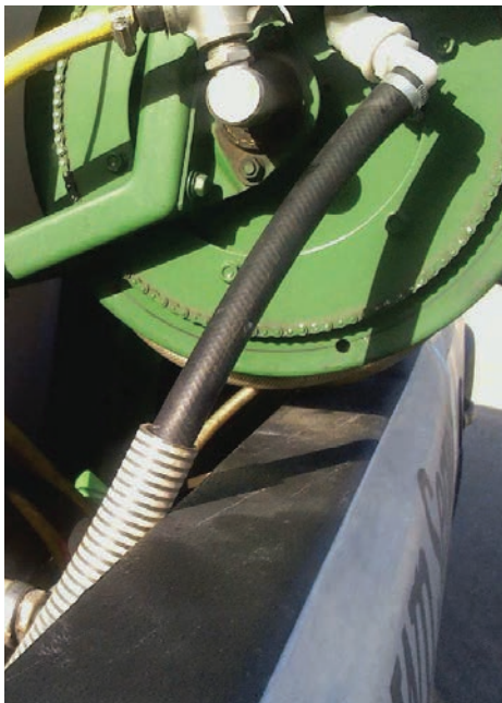
(Top left and right) These hoses have a protective sleeve. (Bottom left) The operator has wrapped a suction hose around a pressure hose to act as a protective cover. (Bottom right) This operator created a barrier between the hose and the metal frame.
