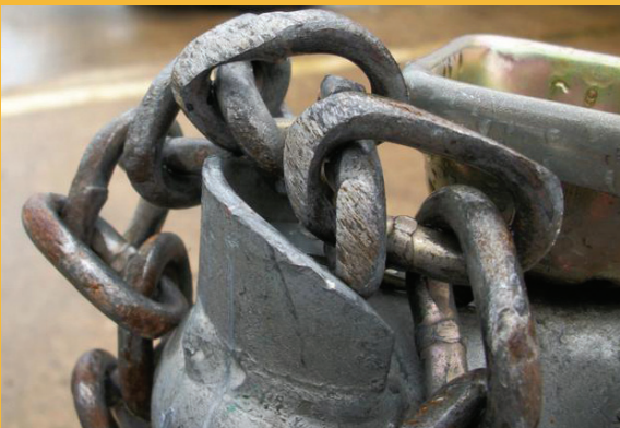
This chain is worn and weak.
