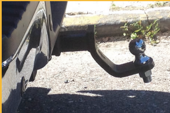
Another hitch with a bent receiver.
