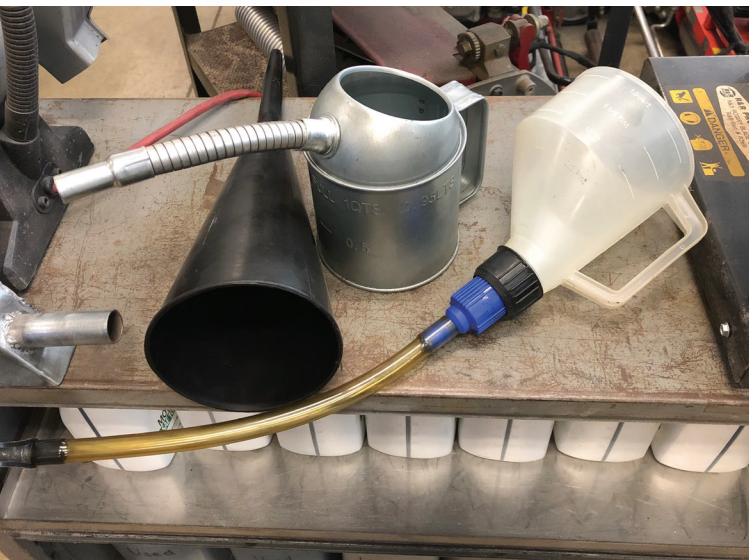
Take care not to introduce external debris from oil fill devices. This may seem like a minor detail, but in fact, it is very important.
