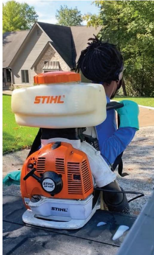
*A full backpack mist blower is heavy. Instead of lifting the blower off the ground, place it on the tailgate and slip the straps over your shoulders.*
