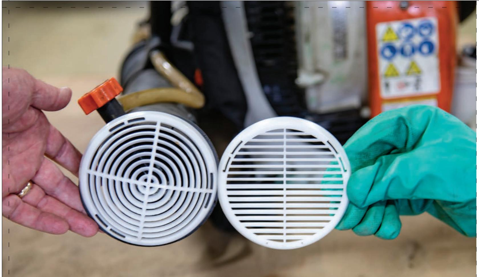
*Applicators can use two types of directional nozzles. The one on the left is the more typical nozzle that blows straight out. Applicators can control the direction the spray travels by the direction of their circular application motion. The nozzle on the right has a plastic outlet cover that points down, which can keep the spray aimed downward.*
