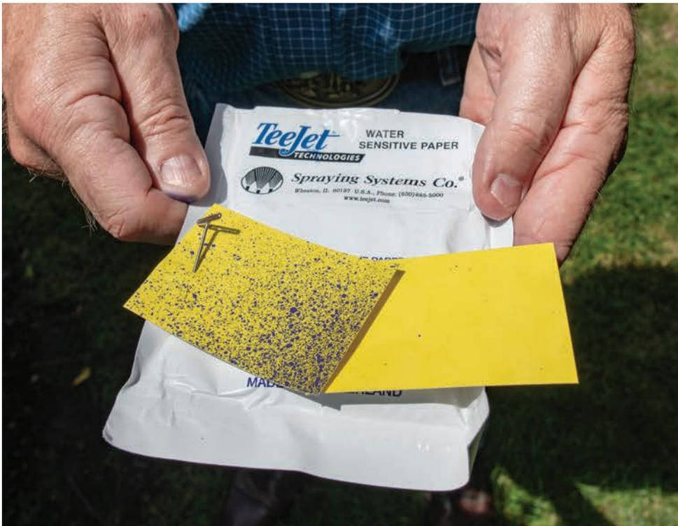
*The many blue dots on the paper show good coverage from spraying near the plant's base. The water-sensitive card inside this tree shows no insecticide spray penetrated the interior. The difference between the coverage was the distance away from what was being sprayed; the farther away, the less coverage within the plant's interior.*
