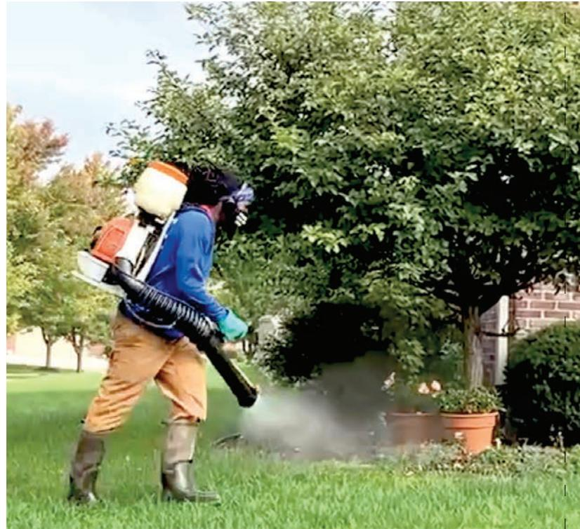
*A backpack mist blower delivers small droplets pushed by air to coat both sides of the leaves.*
