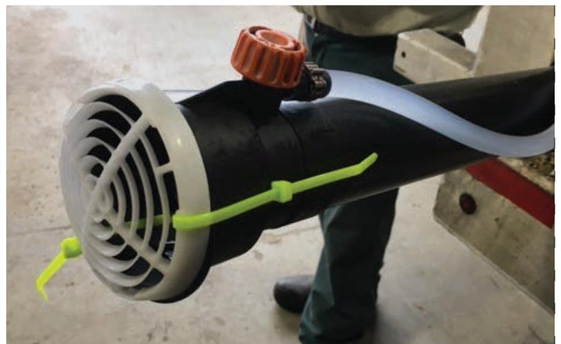
*An example of securing a nozzle onto a backpack mist blower.*
