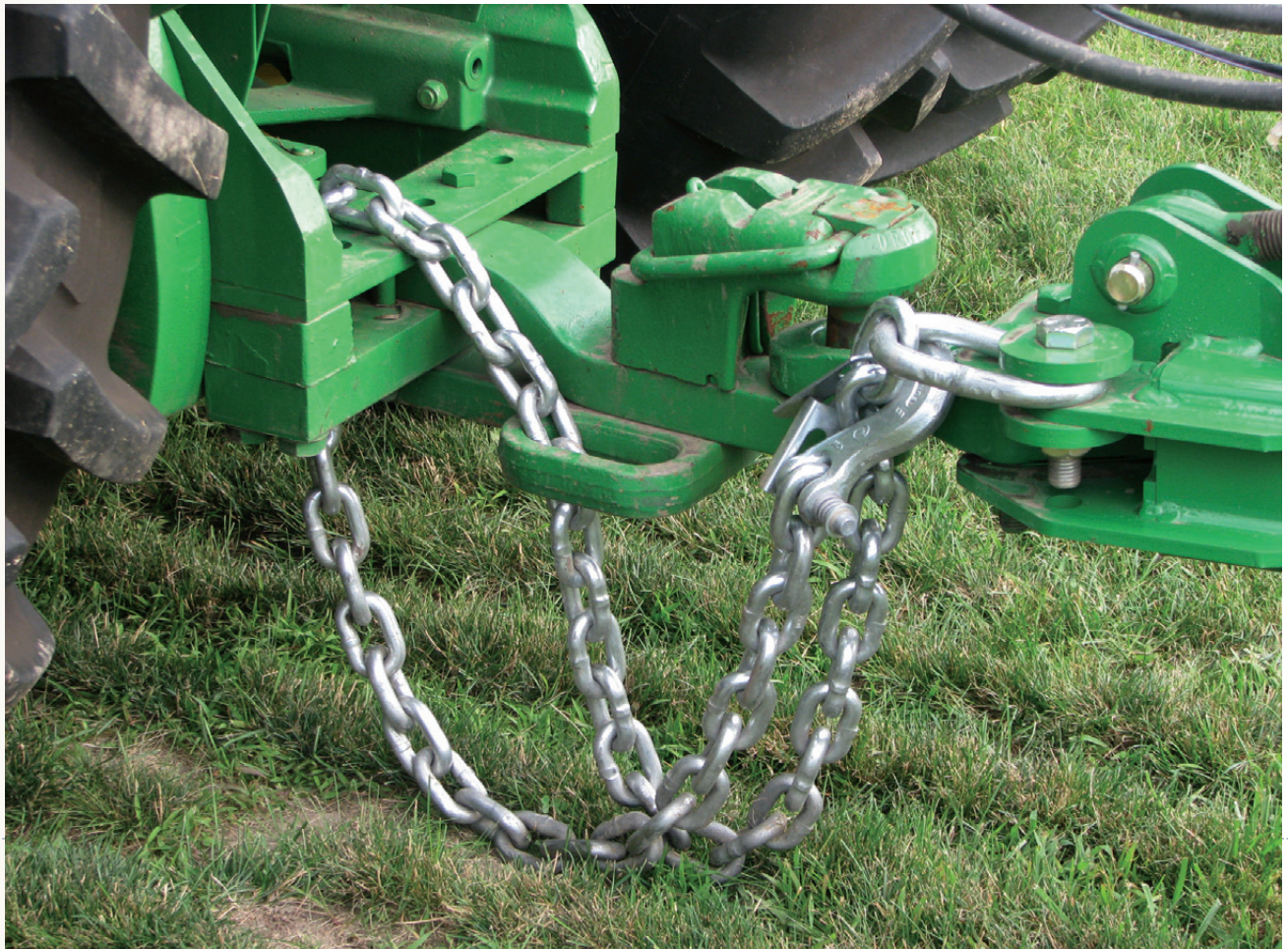
This chain is properly hooked, but needs to have the slack adjusted. One way to do this is to wrap the chain around the drawbar support.
