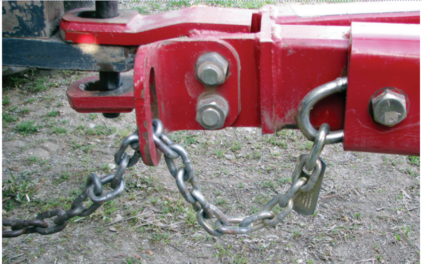
A proper use of the intermediate support, which keeps the chain from dragging.
