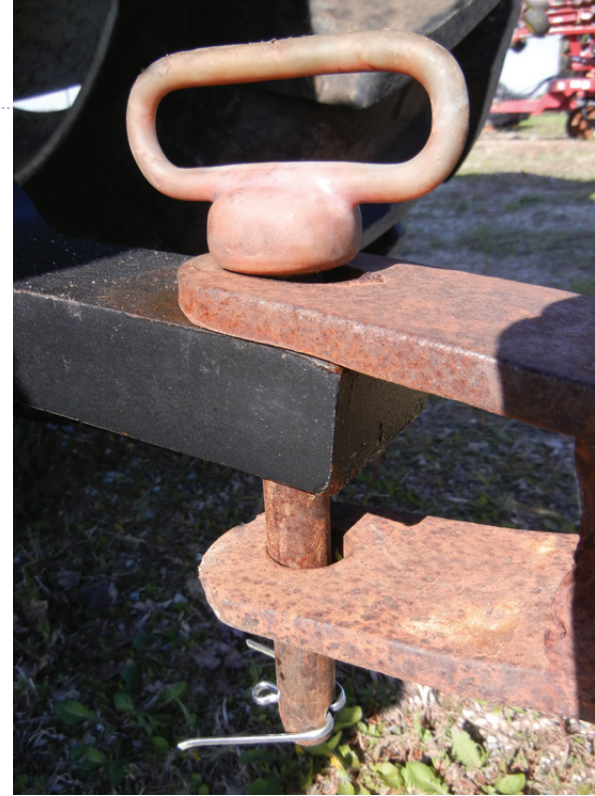
(Above left) A more robust clip in a hitch pin that has less chance to fail. (Above right) A cotter pin can be bent into the hitch pin opening when the tractor and wagon will be hooked for longer periods of time. However, this cotter pin is softer than this safety clip and would fail sooner.
