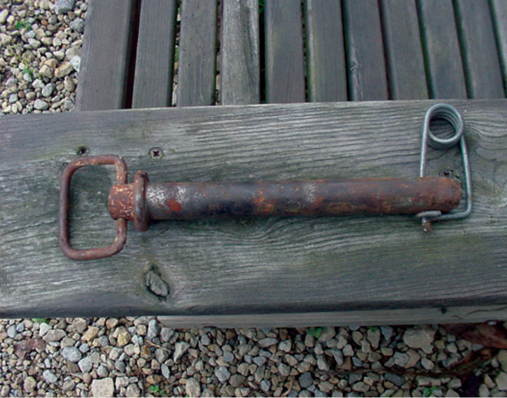
(Above left) A more robust clip in a hitch pin that has less chance to fail. (Above right) A cotter pin can be bent into the hitch pin opening when the tractor and wagon will be hooked for longer periods of time. However, this cotter pin is softer than this safety clip and would fail sooner.
