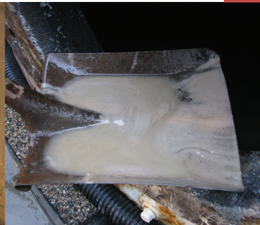
This tank was cleaned six years ago. Materials that are not agitated will salt out, and the residue tends to accumulate around the perimeter of the tank.
