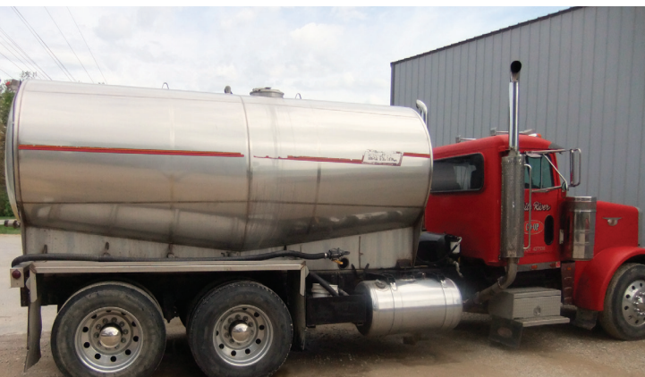
Normally, the number of lids determines how many compartments are in a tank — a stainless tank with a single compartment (top) and one with two compartments (right). Some manufacturers will add a second lid to a single tank for better access to the inside of the tank when cleaning.
