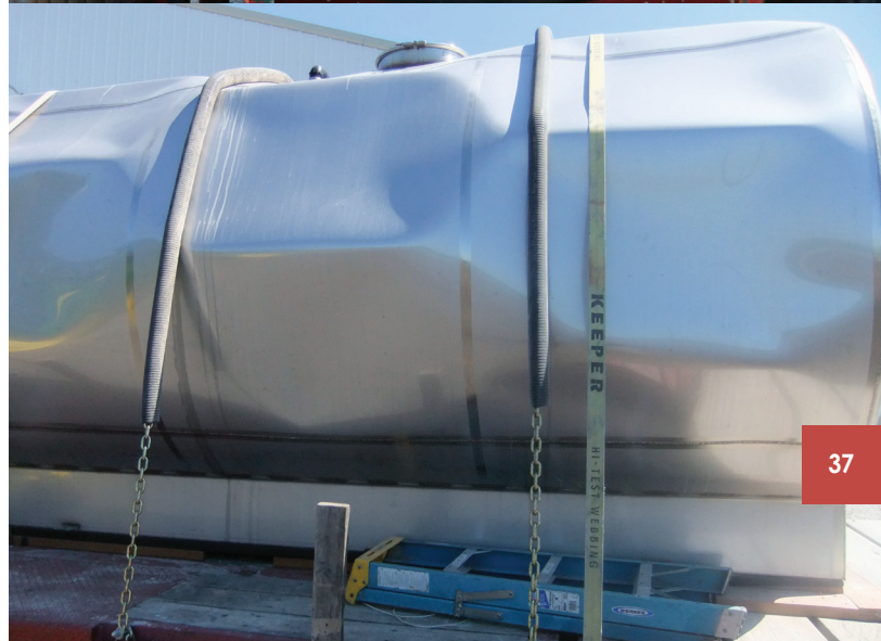
These tanks imploded because of inadequate venting. Tanks implode when you pull liquid out of the tank faster than air can enter the tank. Under the right conditions, even storage tanks can implode.
