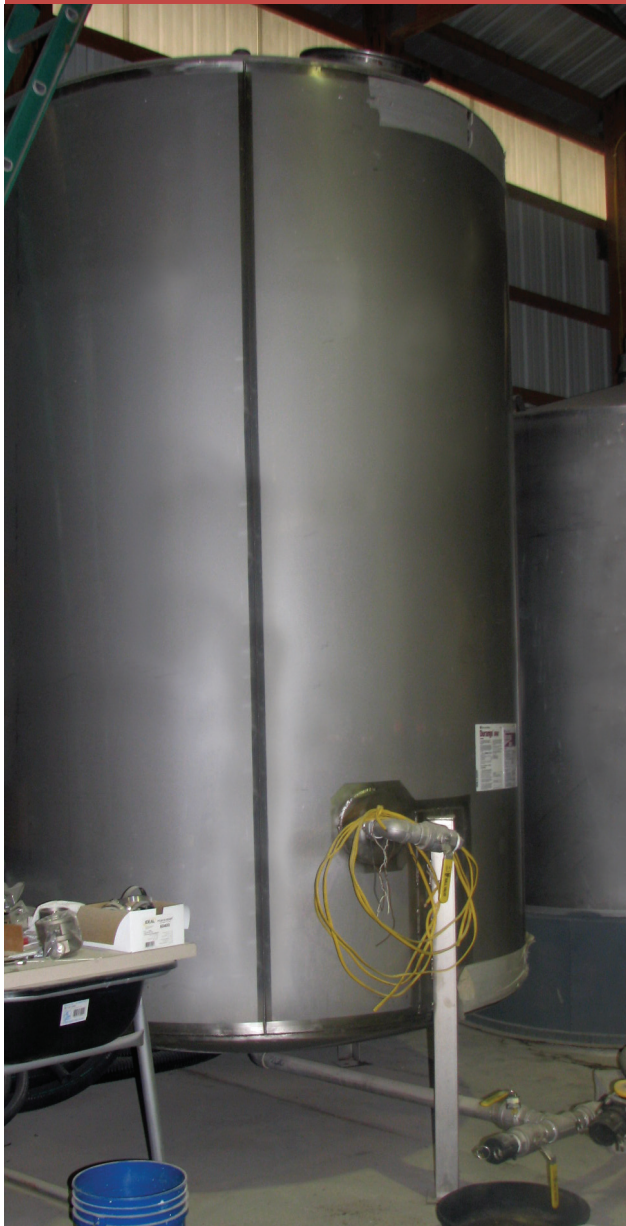
A fitting on the bottom of a stainless tank allows you to empty it completely.
