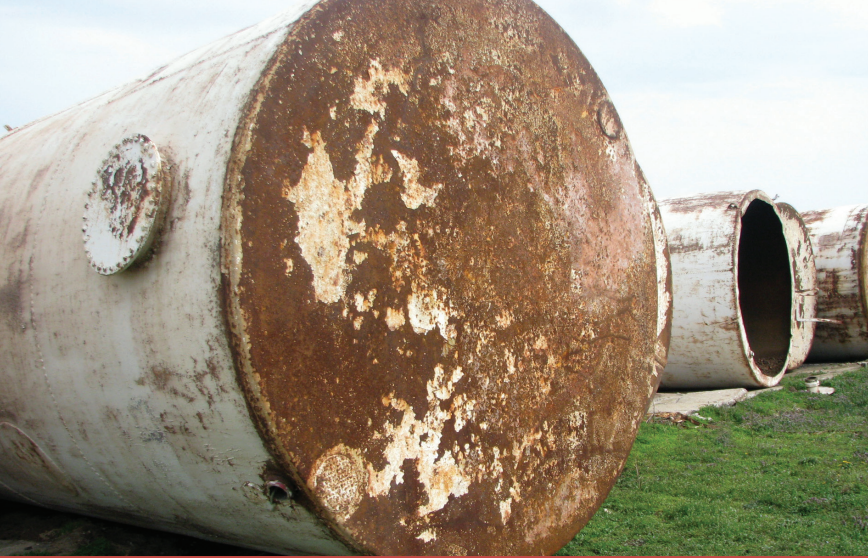
A tank with rivets was probably made before or during World War II. The arrow points to a missing rivet. It is important to thoroughly inspect an old tank like this before you buy it.
