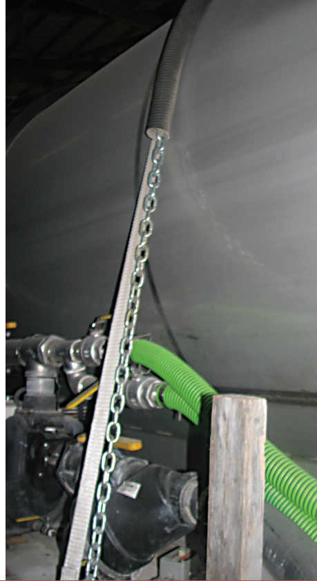
(Top left) This tank has chains directly on it, which could lead to problems. On the other tanks, notice that the chains are run through hoses that help to protect the tanks' surfaces.
