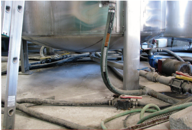
A fitting on the bottom of a stainless tank allows you to empty it completely.
