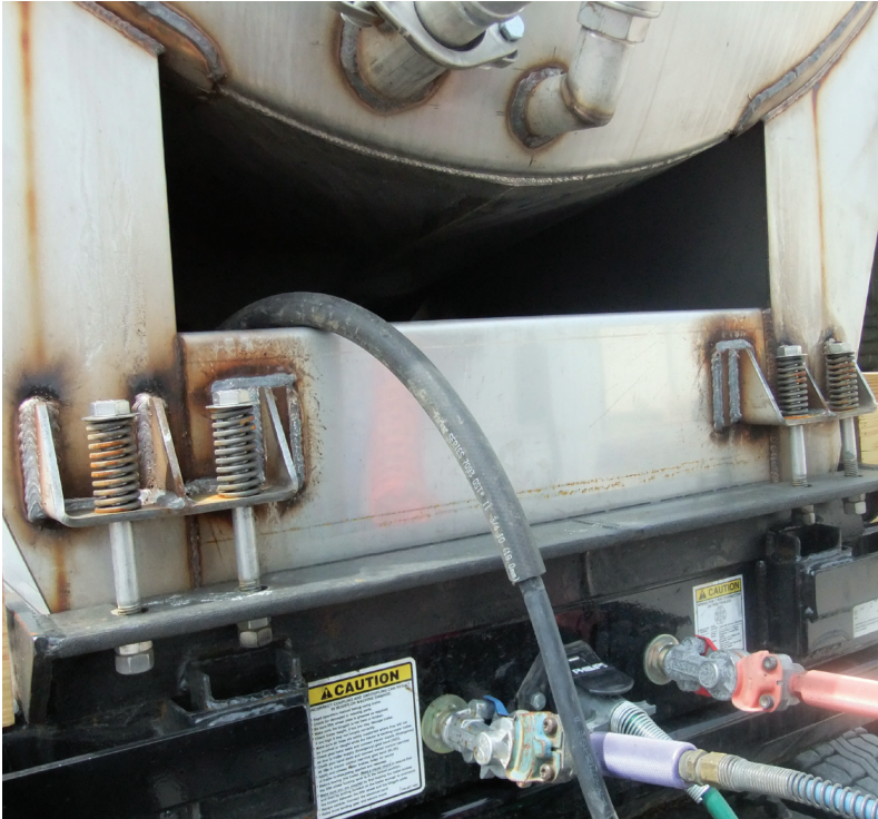
These pictures show the springs and welded metal stops on the outside of a tank.
