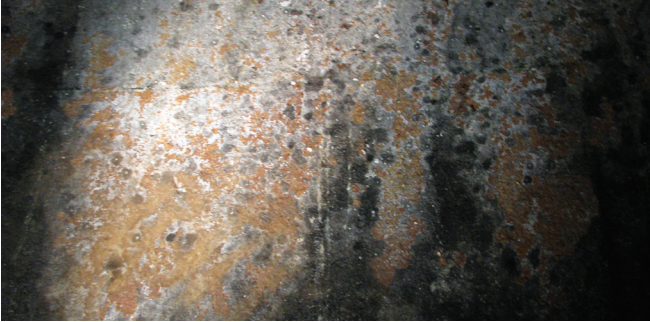
(Left) This tank has a pit. (Right) A close inspection turns up a small crack above a weld.
