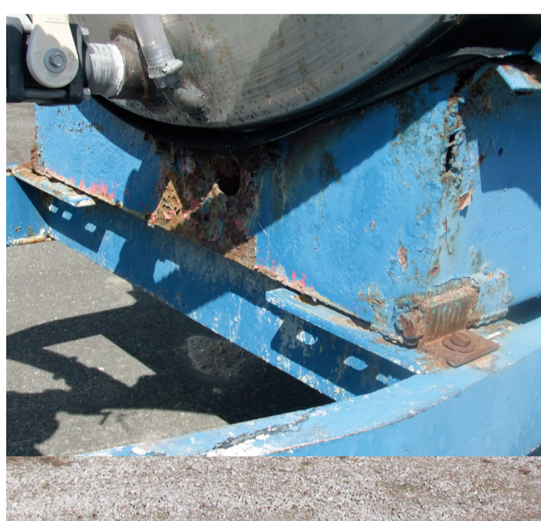
This tank looks like it developed a problem from a leaking line. General corrosion (such as rust) is mainly a cosmetic issue. A tank failure caused by general corrosion is a slow process.
