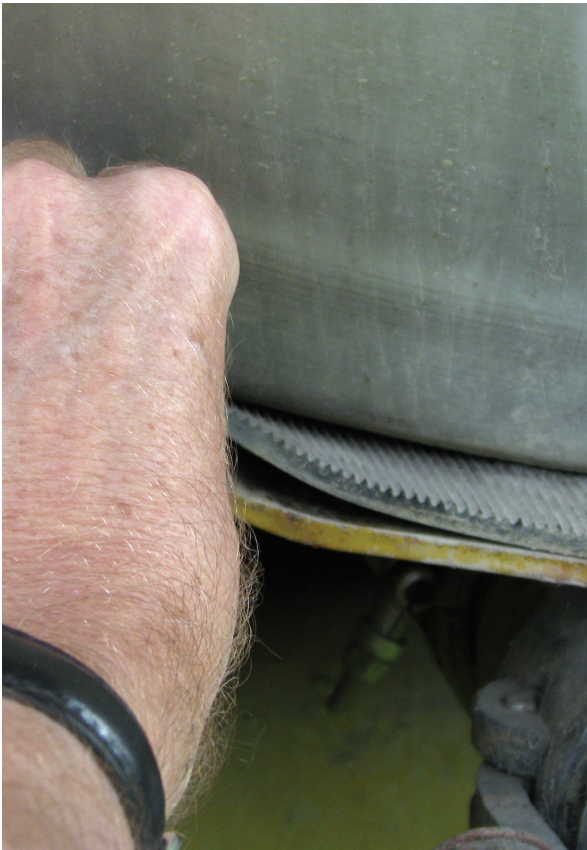
Rubber strips placed between the tank and metal frame help protect the tank from getting holes rubbed in it.
