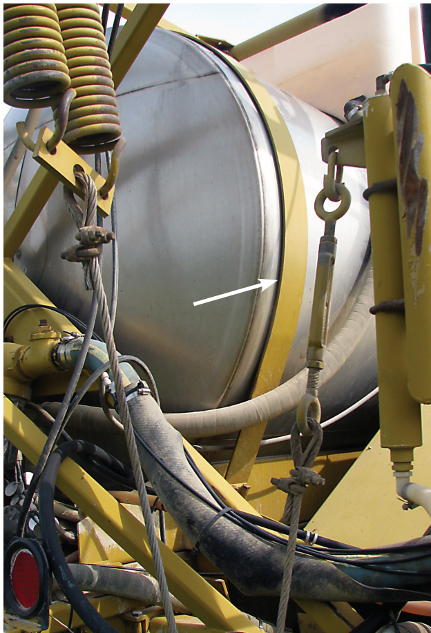
A sight gauge should always have a shut-off valve. This will allow you to open the valve when loading or unloading and to close it to prevent spills while in transit.
