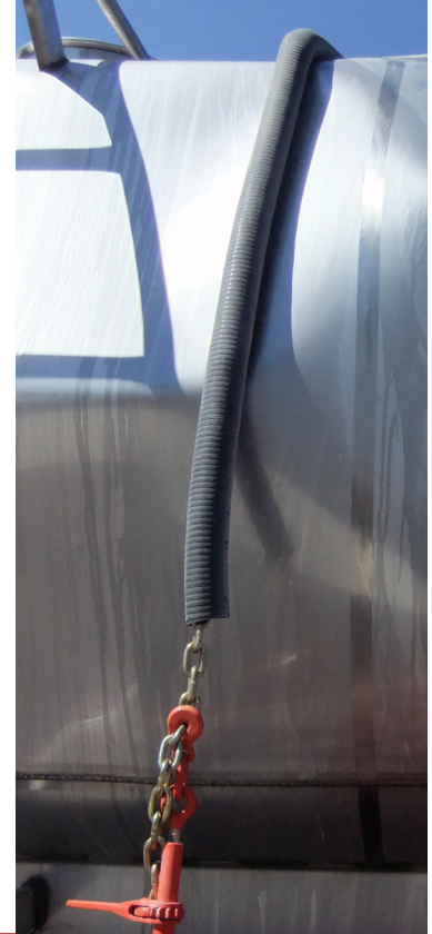
(Top left) This tank has chains directly on it, which could lead to problems. On the other tanks, notice that the chains are run through hoses that help to protect the tanks' surfaces.
