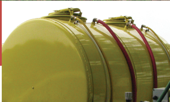
Normally, the number of lids determines how many compartments are in a tank — a stainless tank with a single compartment (top) and one with two compartments (right). Some manufacturers will add a second lid to a single tank for better access to the inside of the tank when cleaning.
