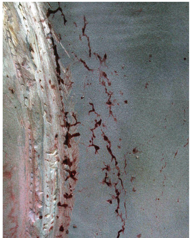
A dye penetrant test makes the metal failure in this tank obvious.
