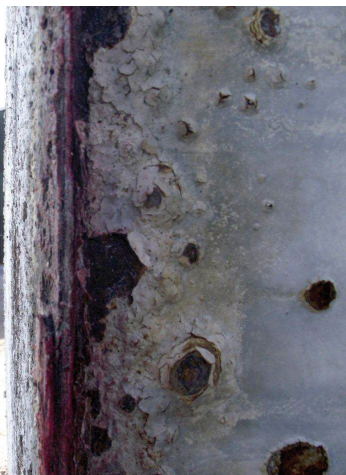
The bottom of this tank is showing signs of corrosion (left). Keep water away from the tank to help reduce corrosion next to the tank (middle and right).
