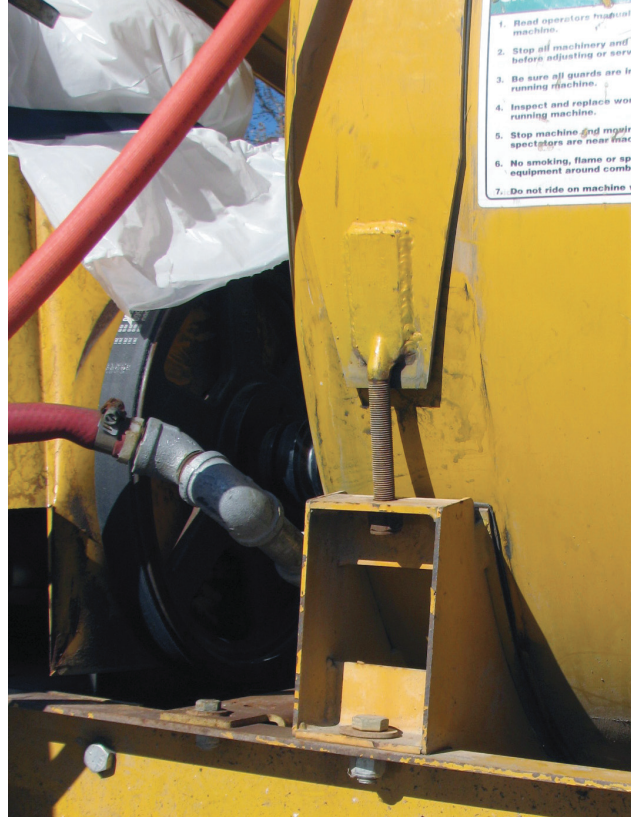
A rubber strip between the tank and bracket or hold down strap will reduce the stresses that can come from twisting and bending.
