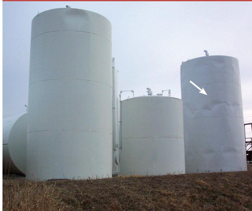
These tanks imploded because of inadequate venting. Tanks implode when you pull liquid out of the tank faster than air can enter the tank. Under the right conditions, even storage tanks can implode.
