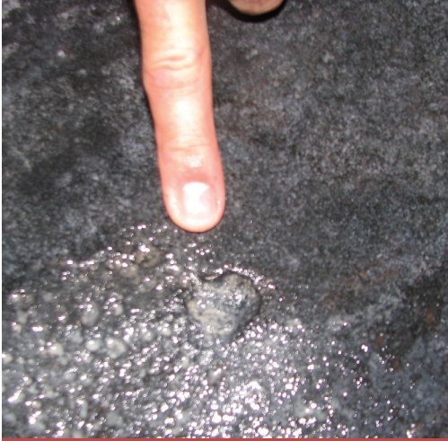
(Left) This tank has a pit. (Right) A close inspection turns up a small crack above a weld.
