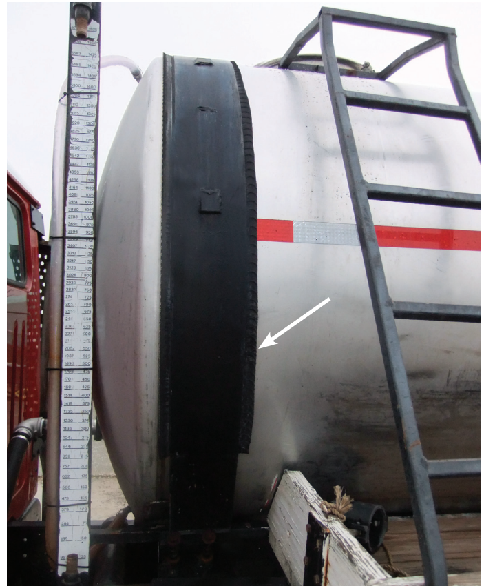
Rubber strips placed between the tank and metal frame help protect the tank from getting holes rubbed in it.
