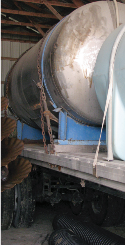
(Top left) This tank has chains directly on it, which could lead to problems. On the other tanks, notice that the chains are run through hoses that help to protect the tanks' surfaces.
