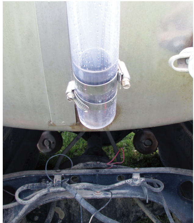
A sight gauge should always have a shut-off valve. This will allow you to open the valve when loading or unloading and to close it to prevent spills while in transit.
