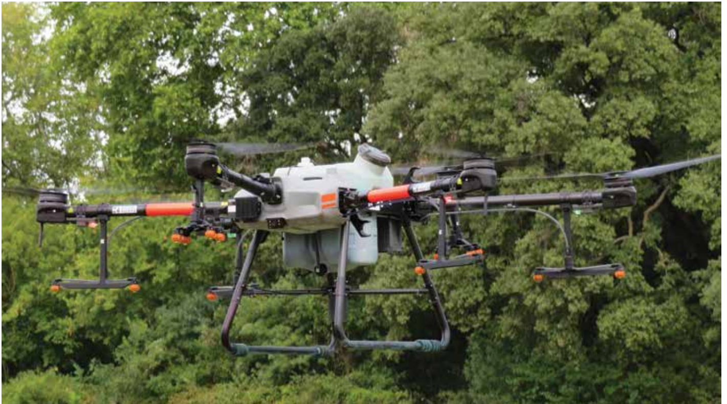
The DJI Agras T30 is a spray drone designed for use by commercial applicators and farmers.
