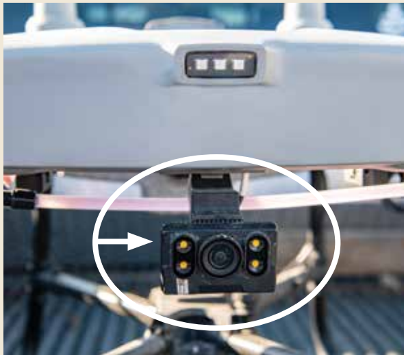
This DJI Agras T10 has a camera in the front and is flanked on either side by an obstacle avoidance sensor.
