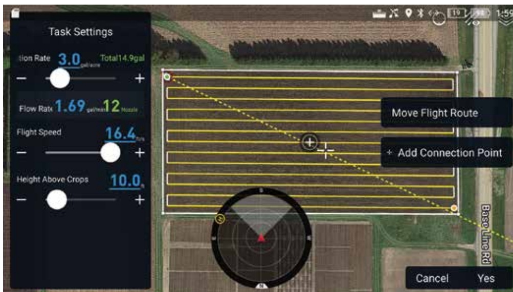
This controller says the drone is applying 3.0 gallons per acre. The only way to know if this is accurate is to measure the flow rate in GPM and convert it into an application rate in GPA.
