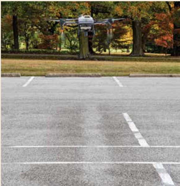
Spraying 5 feet above the pavement is not high enough to deliver an acceptable and uniform pattern.
