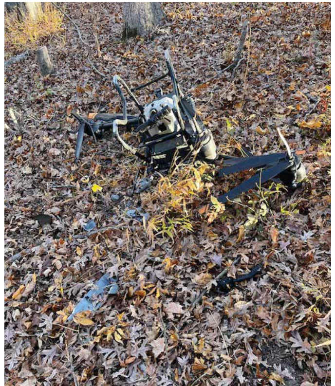
This drone encountered an obstacle while returning to home base with no remote-control signal and paused. The drone hovered until its battery reached a critically low level, and then attempted to land through the canopy of a mature deciduous forest.
