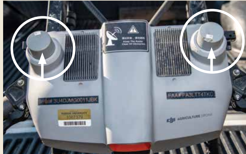
The drone receives a signal from the controller via its two antennae. The two black panels on the side of the receiver allow air flow that helps keep the hardware in the drone from overheating.
