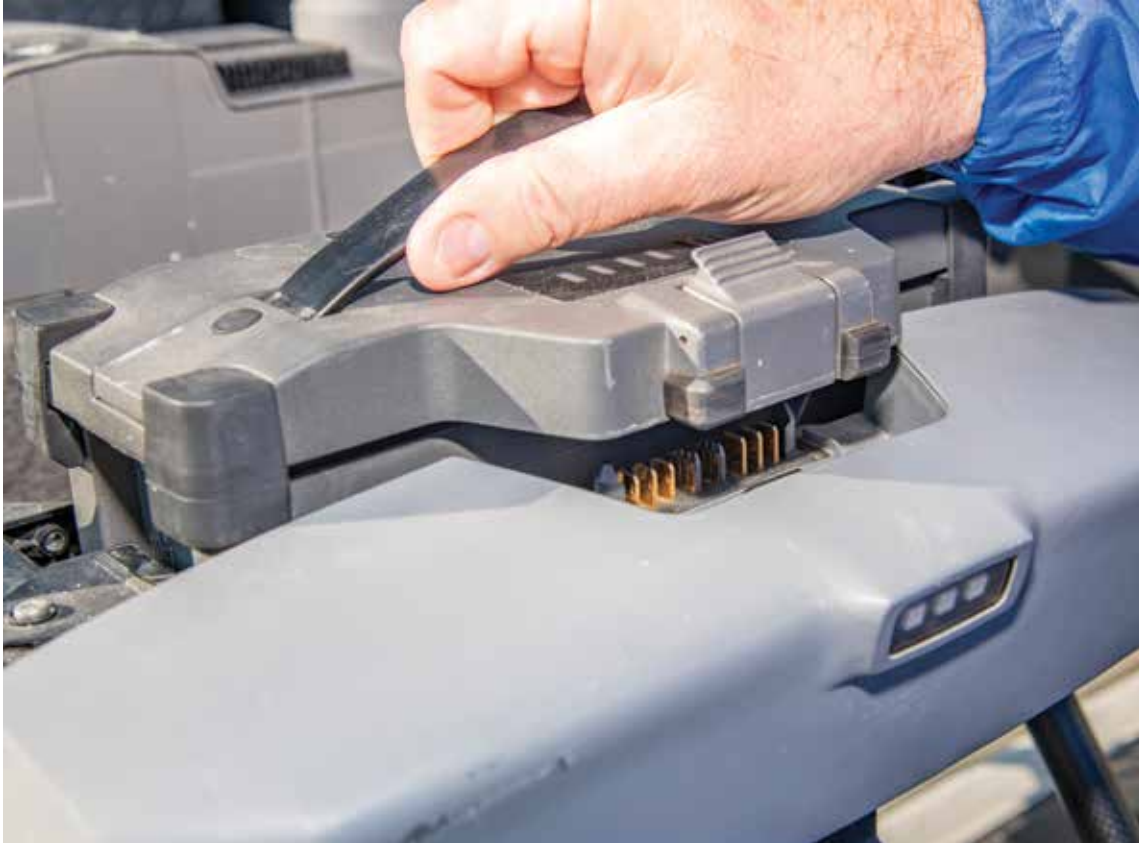
When batteries are not in place, electrical components are exposed and are at risk for damage.
