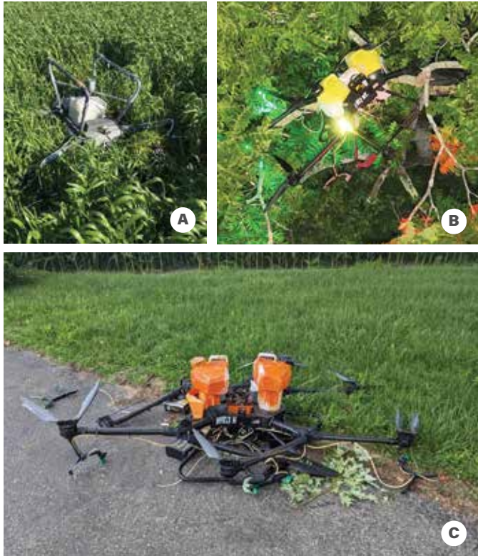
Photos A, B, and C. Unexpected landings can place drones into unwanted and unsafe landing zones, which may substantially damage drones.
