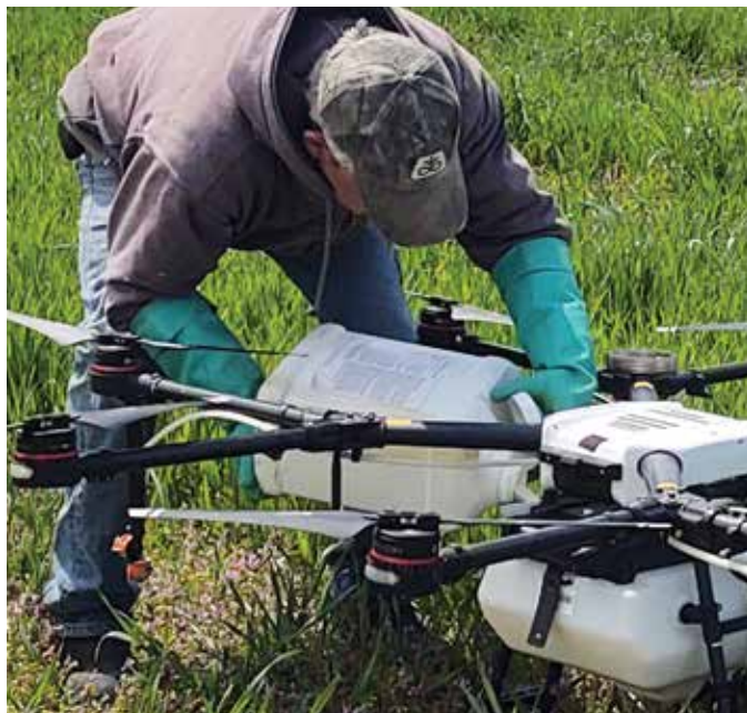
It is important to wear chemical-resistant gloves when handling spray drones because the aircraft exterior will have pesticide residues.
