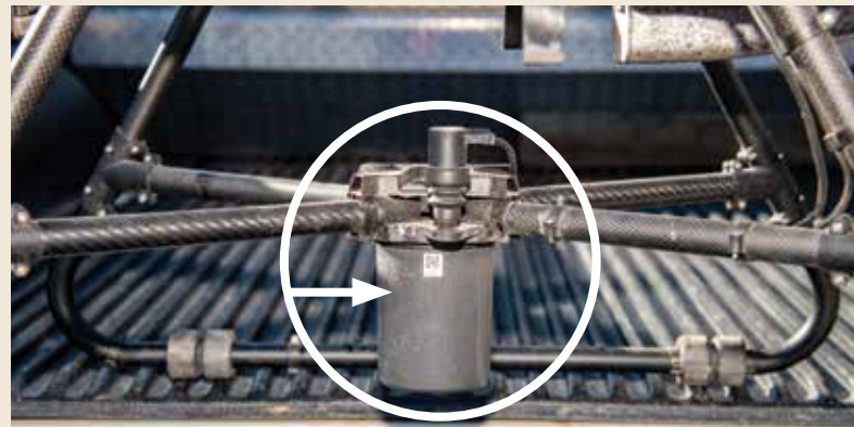
This device is called an omnidirectional digital radar system. It measures the altitude that is recorded on the controller.
