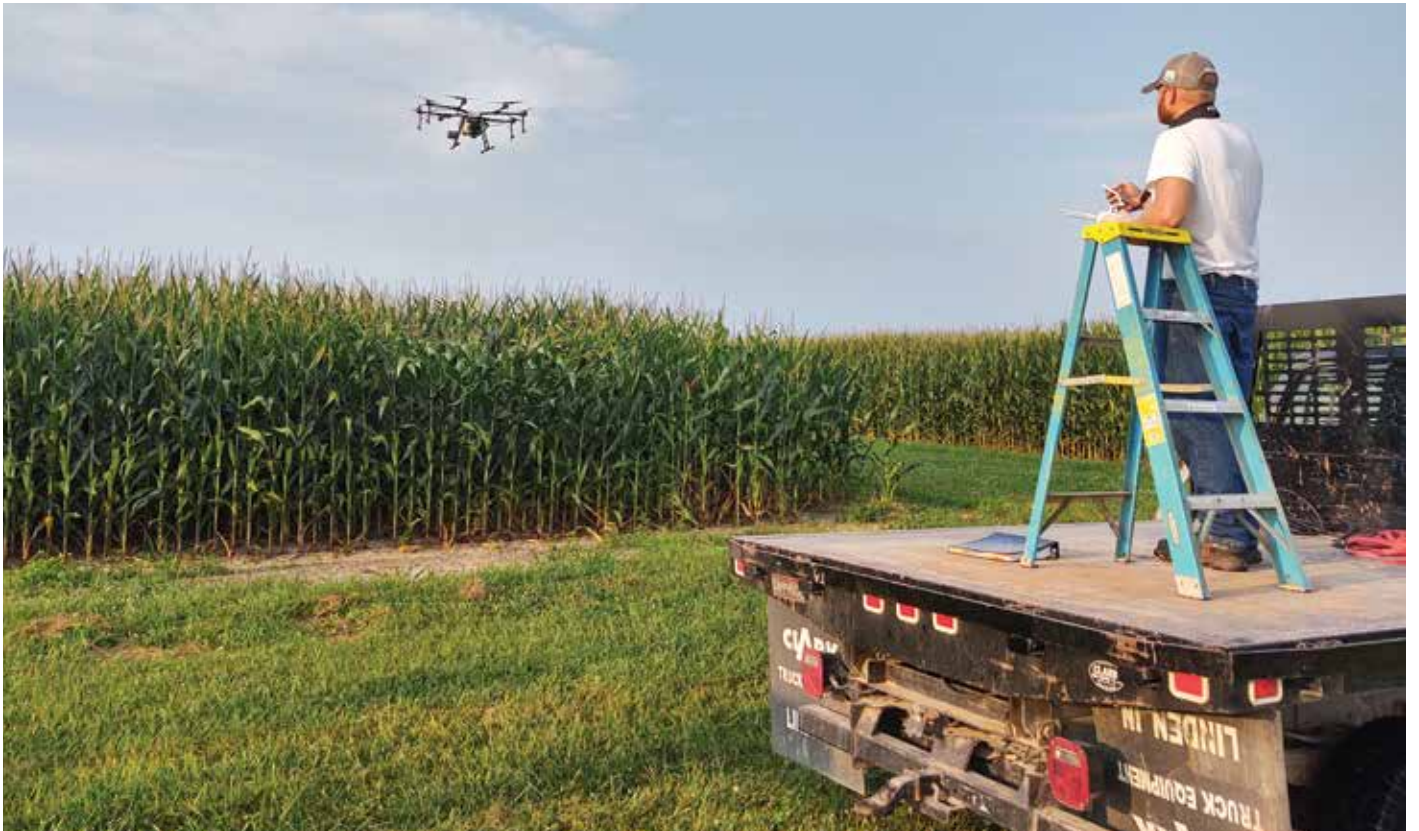
This pilot placed a ladder on a flatbed trailer to improve line of sight. Safe ladder use now becomes an issue that must be addressed.
