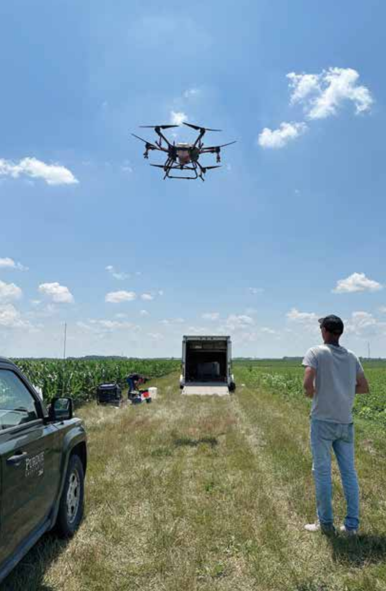
Nozzle type, spray height, and carrier volume are some of the factors researchers are evaluating to determine optimal spray drone applications.
