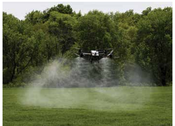
This photo shows the spray distribution and swath emitted from a DJI Agras T40 using rotary atomizer (spinning disc) nozzles.
