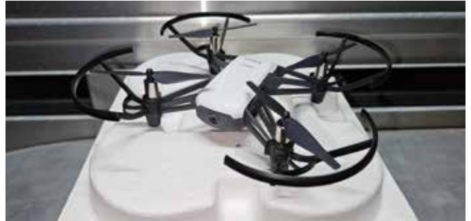
This is an example of a drone that weighs less than 0.55 pounds and is exempt from many FAA regulations.
