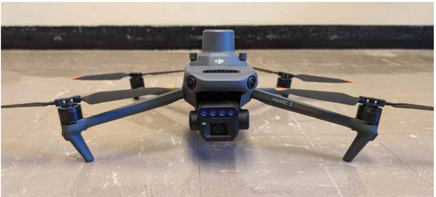
This DJI Mavic 3M has a multispectral camera, which can capture green, red, red edge, and near infrared bands. The larger gray top is the RTK receiver.
