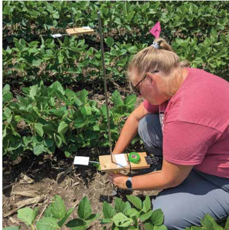
Researchers are examining ways to better understand the spray deposition and efficacy of spray drones to make proper application recommendations.
