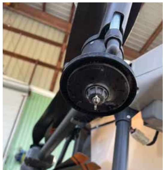
Examples of rotary atomizers equipped on several new drone models.
