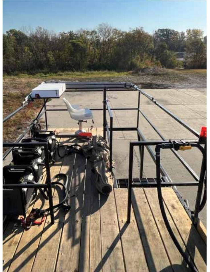
Highly specialized trailers can support spray mixing, loading, battery charging, and elevated observing. In addition, they can provide adequate room for safely landing and walking around drones for inspections and repairs between flight missions.
