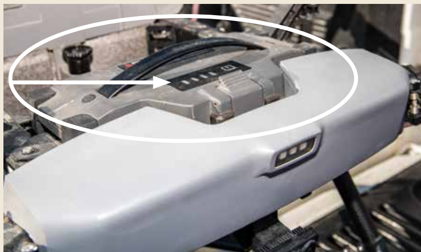
This device is called an omnidirectional digital radar system. It measures the altitude that is recorded on the controller.
