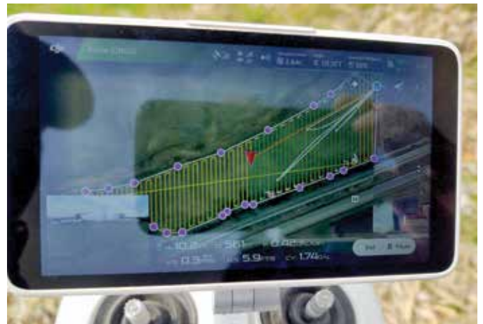
This is an example of the software available with many drones. This image shows an application in progress after the operator developed a detailed flight plan. Yellow lines indicate the drone's flight paths. Each purple dot is a waypoint that indicates a change in the application boundary, which signal the drone to change direction.
