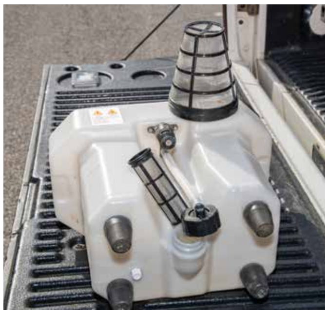
Many drone solution tanks have removable strainers that allow for easier cleaning.
