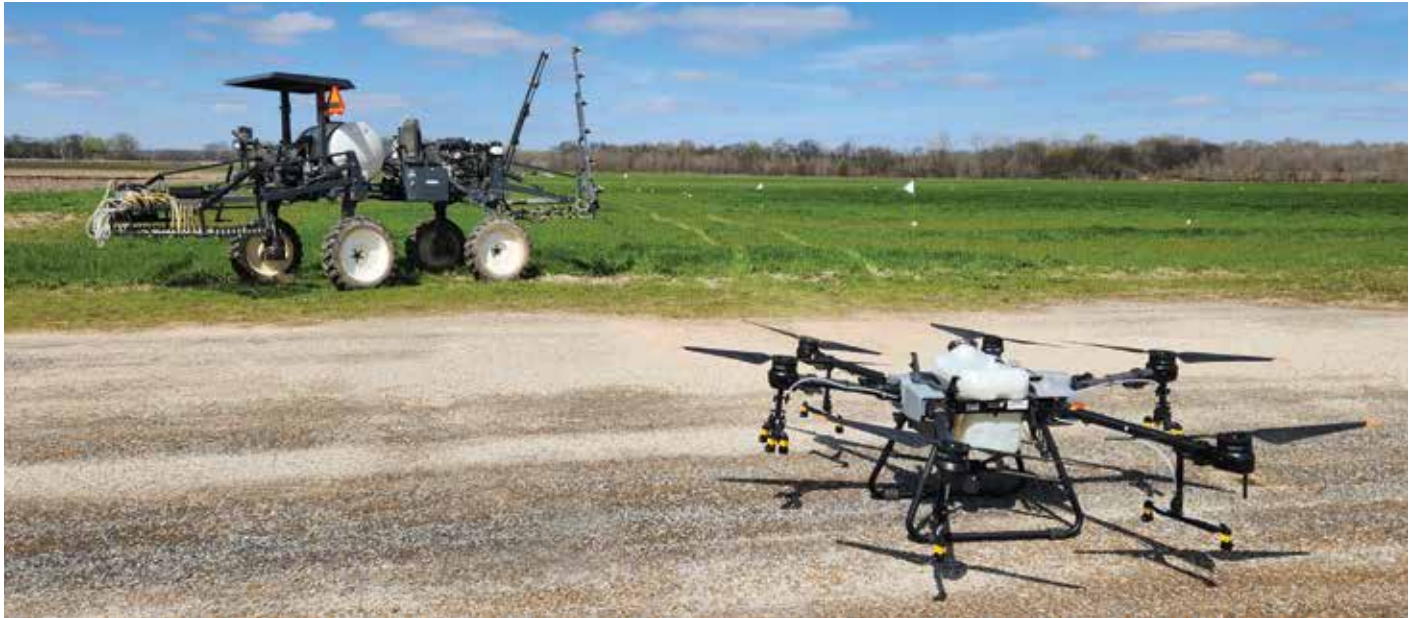
Spray drones are unique pieces of application equipment compared to ground boom equipment. Researchers are evaluating drones to find optimum use practices.
