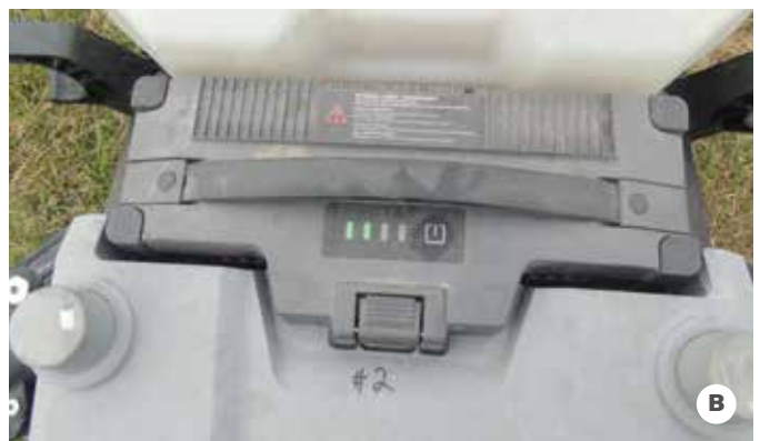
Most batteries have lights that indicate how much battery life remains. (A) These four lights indicate the battery is fully charged. (B) This battery has used up half of its battery charge.
