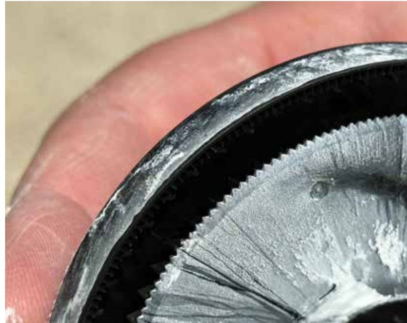
The small grooves in the spinning discs act as tiny channels that distribute liquid while it is dispersed. The liquid eventually forms droplets as it leaves the spinning disc. The grooves wear with more abrasive materials. Always carry spare discs to quickly replace them in the field.
