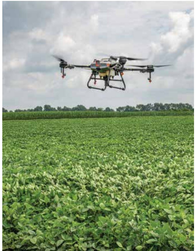
One of the many differences among drone models is how the spraying systems are equipped. This drone is equipped with conventional nozzles underneath the spray rotors.
