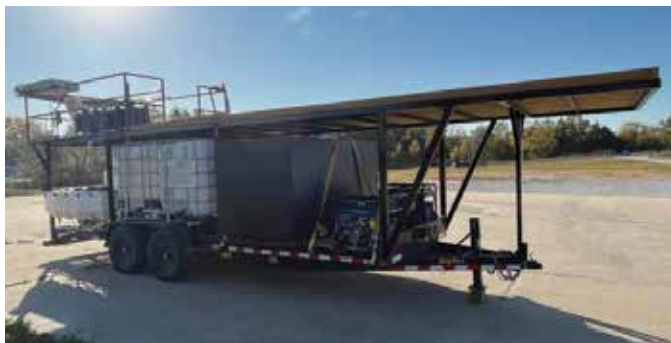
Highly specialized trailers can support spray mixing, loading, battery charging, and elevated observing. In addition, they can provide adequate room for safely landing and walking around drones for inspections and repairs between flight missions.
