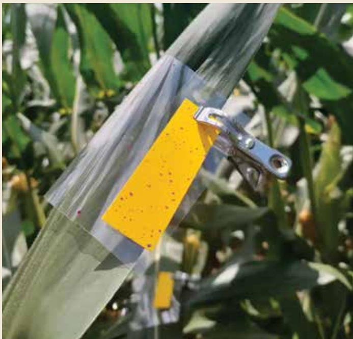
This photo shows a spray width testing card showing deposition after being sprayed by a drone.
