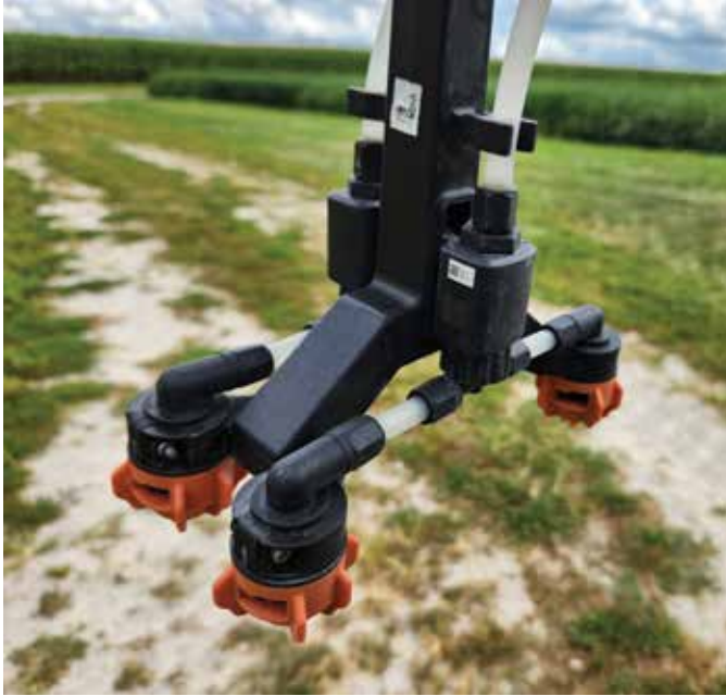
Drones are often equipped with flat-fan nozzles, but the spacing and orientation can be very different from traditional application equipment.
