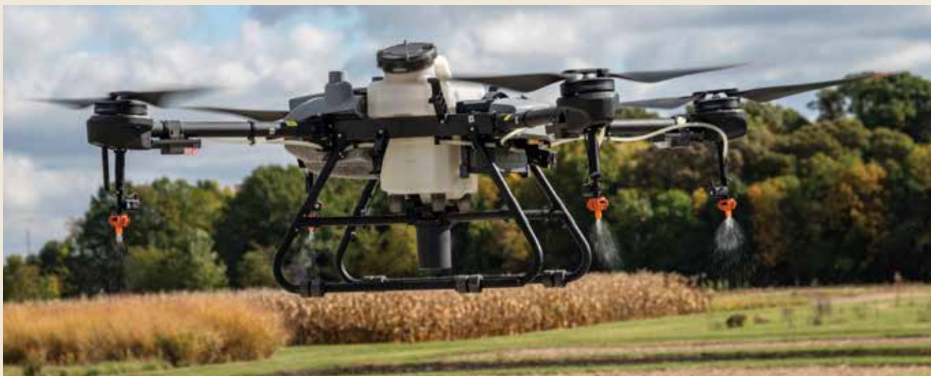
This drone has four nozzles. When flying autonomously, only the nozzles in front of the travel direction turn on for spraying. In other flight mode types and higher application rates, the drone can turn on additional nozzles.
