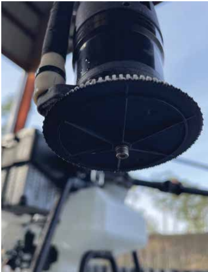
The rotary atomizer (spinning disc) nozzles (like the ones shown here) can create a very uniform droplet size distribution, but more research is needed to fully validate their capabilities on spray drones.
