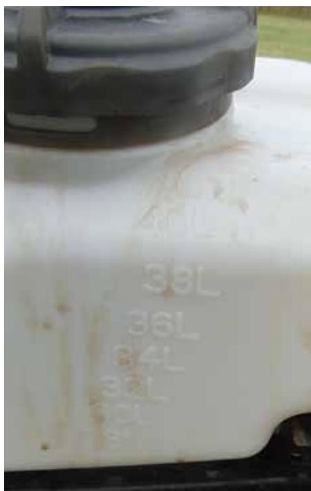
Several spray tanks have labels that indicate different volumes, which can be helpful for accurate mixing. This 38-liter tank is equivalent to 10 gallons.
