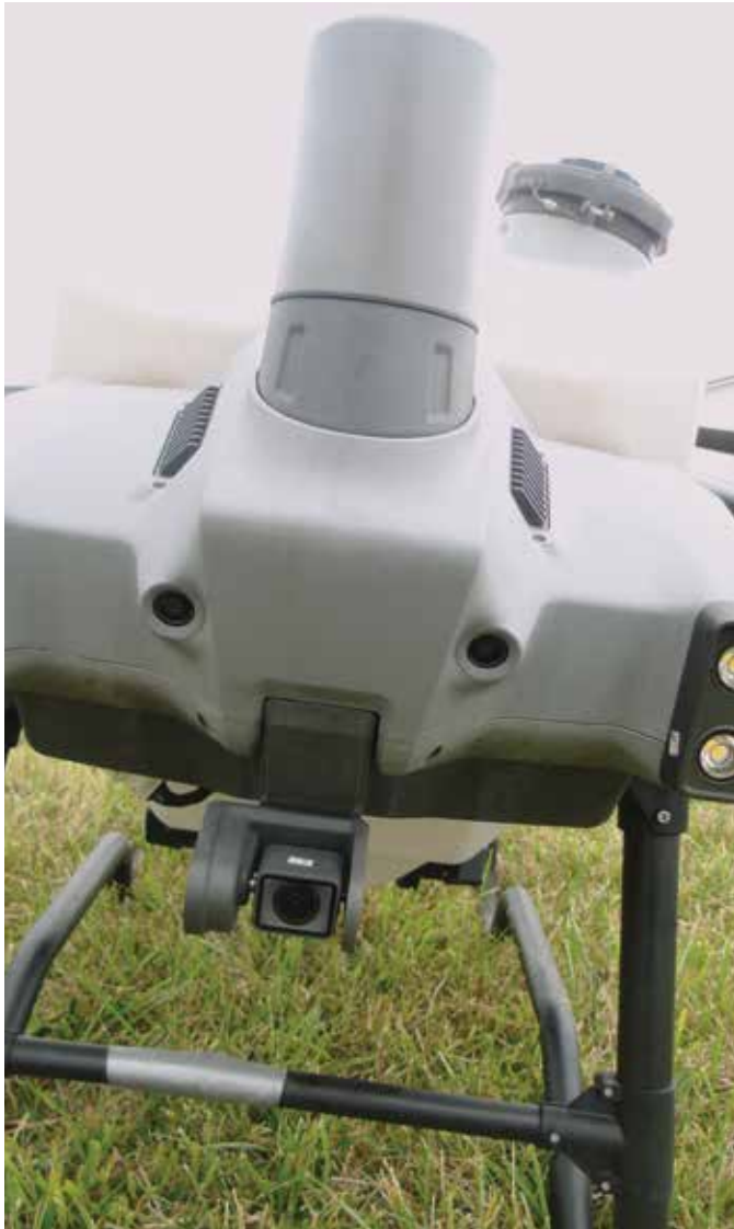
Cameras on spray drones provide real-time visuals of the approaching terrain, crop, and other obstacles during applications.
