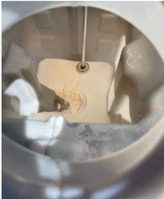
An example of incompatibilities between glyphosate and 2,4-D when mixed in low volumes of water.
