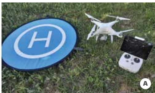
(A) A landing platform, such as the one shown here, can provide a solid base from which to operate a small drone. (B) However, application drones are much larger and require larger landing pads.
