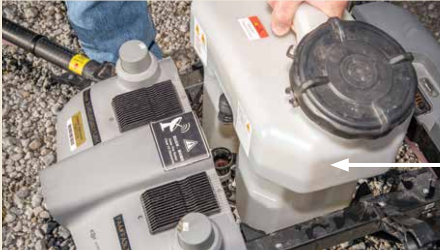
This drone's tank holds 2.5 gallons.
