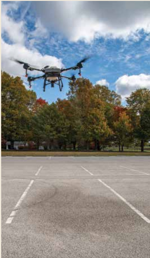
A drone spraying 10 feet above pavement.
