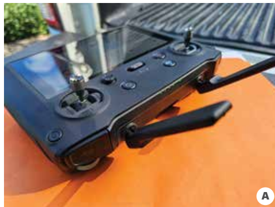
(A) This photo shows the antennae on the controller. (B) This photo shows antennae on top of the drone that receives the signal from the controller.
