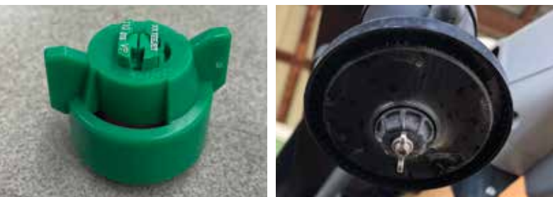
Some spray drones are equipped with common ground equipment nozzles (such as the XR nozzle to the left); however, these nozzles have much smaller orifice sizes than commonly used with ground applications. More modern spray drones use rotary atomizer (spinning disc) nozzles, like that observed on the DJI Agras T40 (right).
