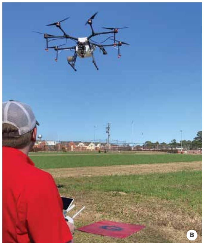
(A) A landing platform, such as the one shown here, can provide a solid base from which to operate a small drone. (B) However, application drones are much larger and require larger landing pads.
