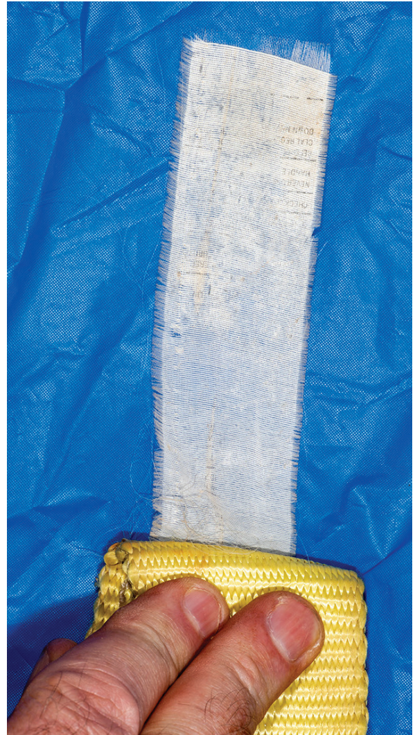
This tag is unreadable. Law enforcement will allocate a WLL of 1,000 per inch of width when tags cannot be read. This 2-inch strap would receive a WLL of 2,000 pounds.
