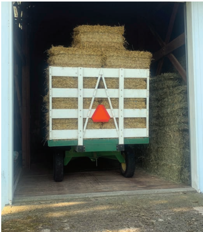
This wagon has a slow-moving vehicle sign clearly visible to warn drivers to slow down. Make sure to replace signs when they fade and become less reflective.
