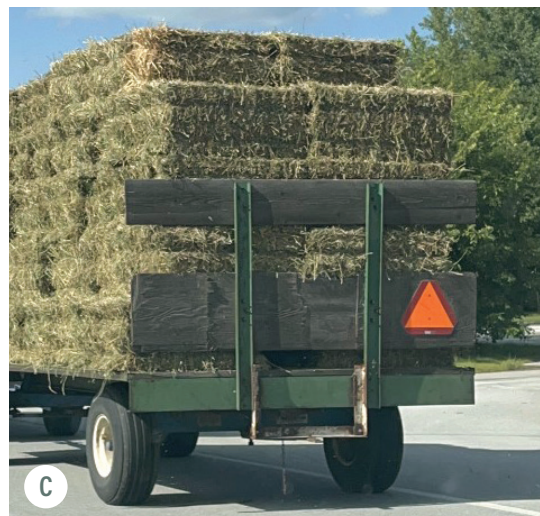
(A) This slow-moving vehicle sign is perfectly placed on the wagon. It is centered both top to bottom and side to side. (B and C) This operator made a good start by placing signs on the back of each wagon. However, the sign on the lead wagon is too high (B) and the sign on the trailing wagon is too far to the right (C).
