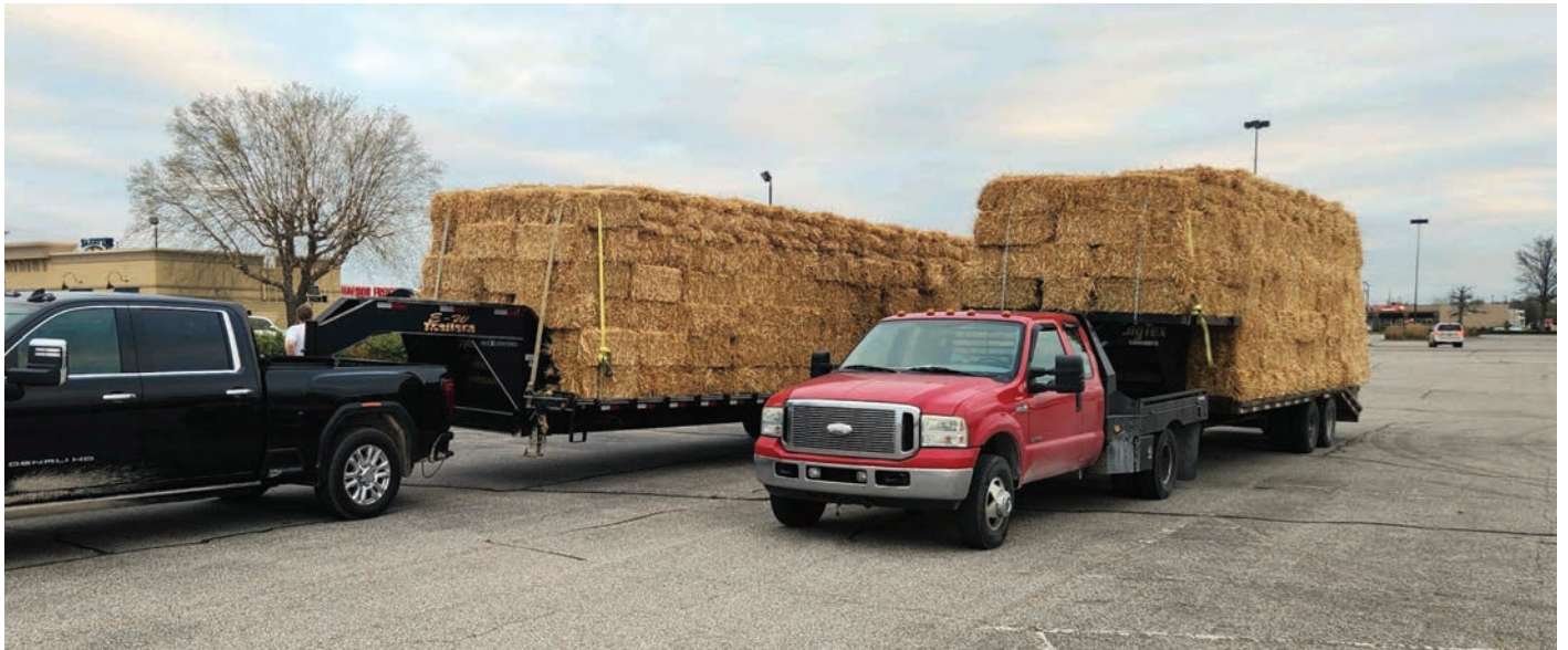
Properly placed straps that run across the top of a load may secure bales from shifting from side-to-side.
