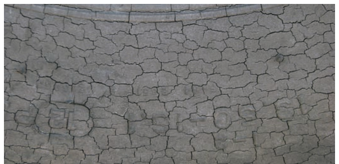
Worn tires can easily blow while hauling a heavy load of hay and straw.
