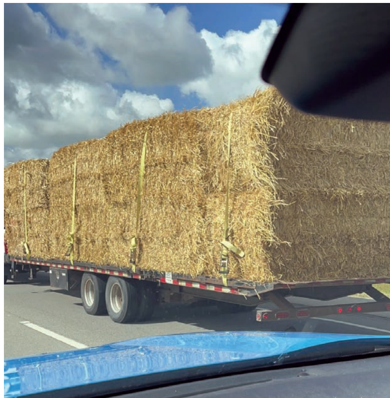
Having enough straps on the side of a load will help prevent bales from shifting and falling onto the highway.
