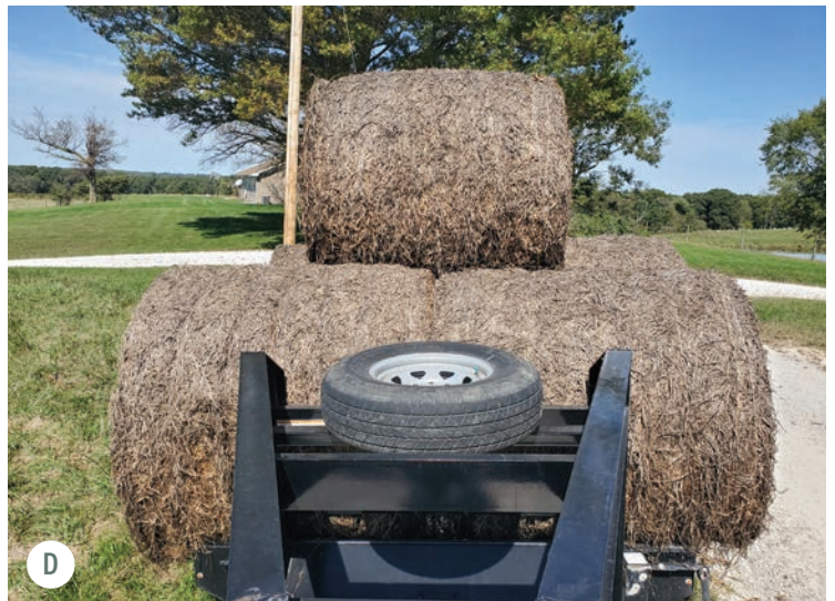
(A, B, and C) These photos show protective structures at the front ends of trailers. (D) While this trailer has a protective device, stacking hay above it will not prevent the top layer from moving forward.
