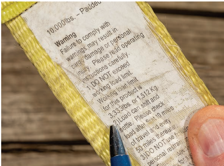
The tag on this strap shows its WLL is 3,333 pounds.
