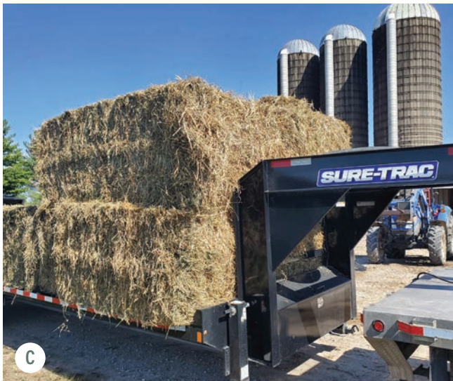
(A, B, and C) These photos show protective structures at the front ends of trailers. (D) While this trailer has a protective device, stacking hay above it will not prevent the top layer from moving forward.
