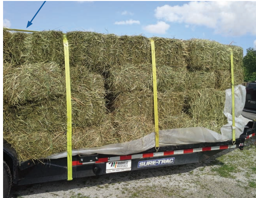
This multi-layer stack of hay will have enough straps running from side-to-side, but it is short one strap on top running from front to back. The alternative load securement method requires two straps running parallel to the trailer (see blue arrow).
