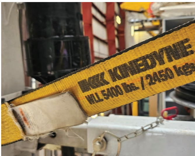
Straps that stencil the WLL onto the webbing assures that you always know the actual value is always known.
