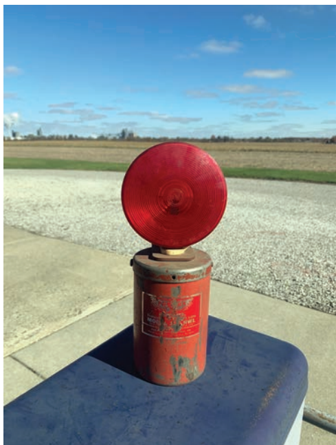
This is a battery-powered warning light with a 9-volt canister flasher.
