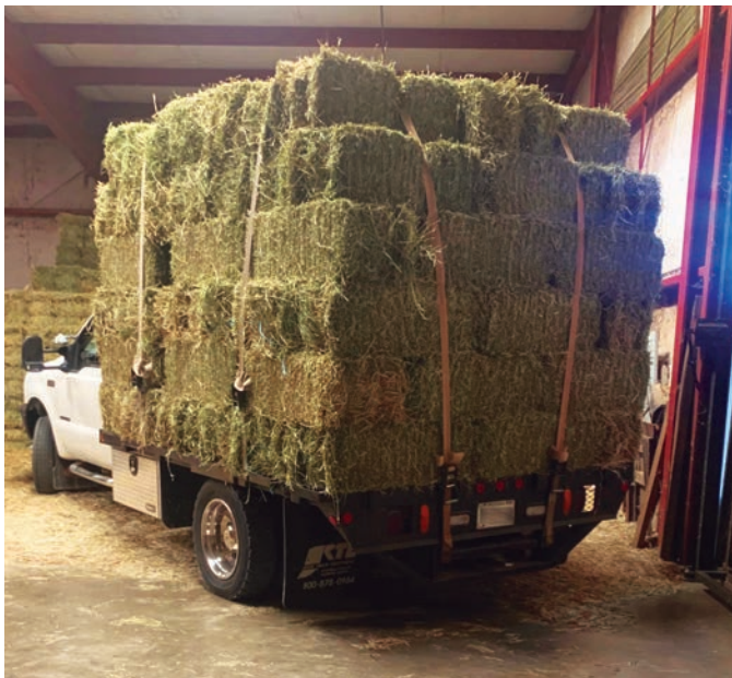
Combining straps going across the width and length of the load offers maximum security from moving left to right and front to back. Any load of small square bales you transport on a roadway should have the front and back row strapped left to right to keep the air from blowing them apart.
