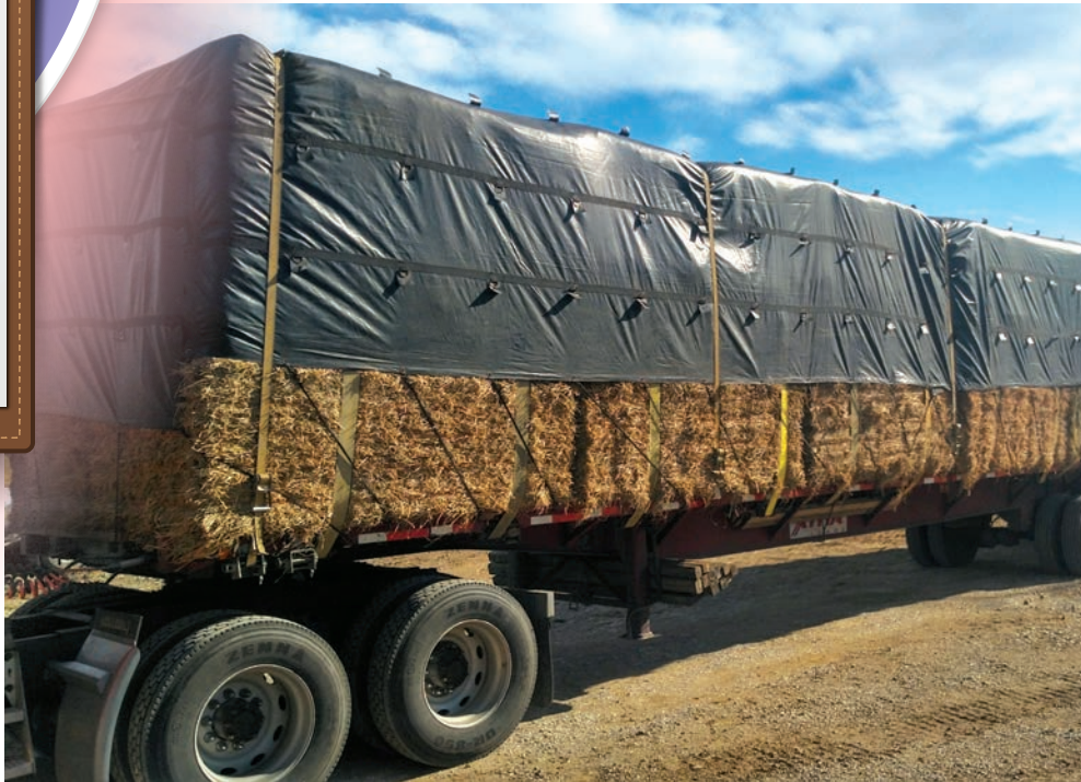
Although this load is not completely tarped, the tarp does keep the winds from blowing most of the loose material off the trailer.
