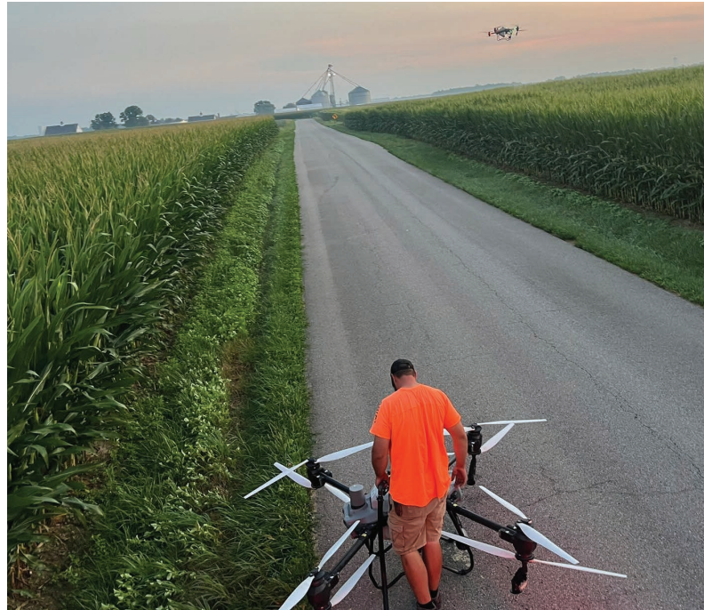
Wearing high-visibility orange is important when operating on or near roads. At least this person has on a high-visibility shirt and glasses on this photo, but they aren't wearing PPE. Both PPE and visibility are part of any good operation.
