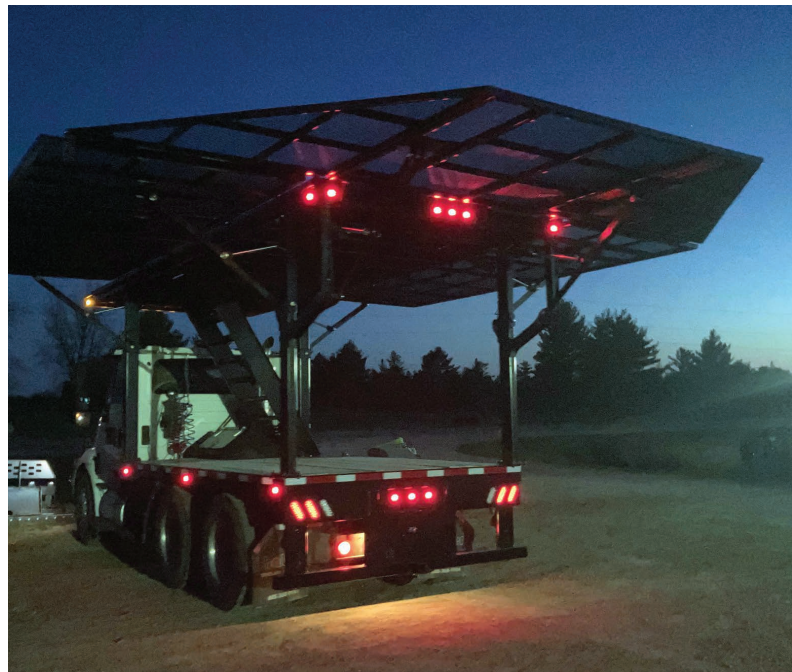
The wide deck allows for plenty of workspace for refilling the drone and swapping batteries. Red lighting helps to reduce the effect of light blinding someone during night operations.
