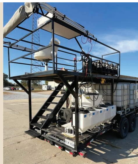
A series of small white totes are part of an auto-mixer. Each tote can contain a specific pesticide that can be metered into the water line running to the application drone.
