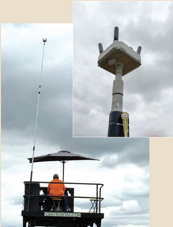
A pilot seated at the workstation. The taller pole allows for the relay to keep a better connection with the drone in fields with less visibility.
