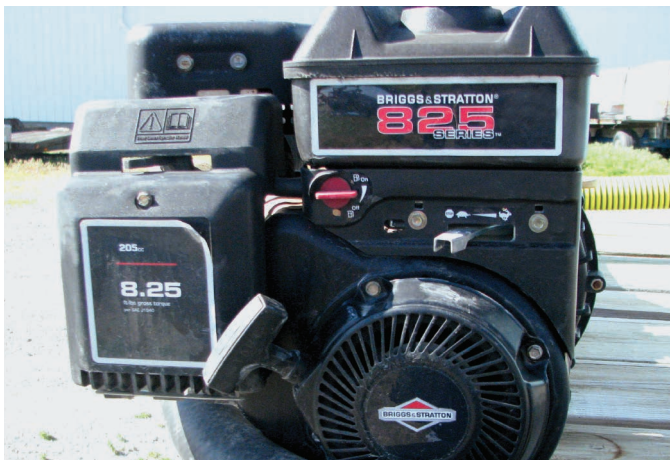
The manual indicates this Briggs and Stratton gas engine has a gross horsepower rating of 8.25 and a net horsepower rating of 6.5.
