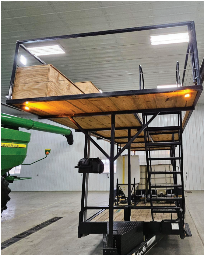
Lighting is affixed to this trailer to help drone operators conduct nighttime operations. Guardrails on the top deck help keep the operator from falling off and may be an OSHA requirement for your operation.
