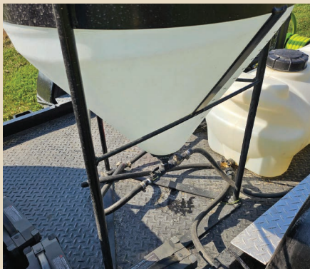
A pesticide can be added directly to the spray tank or to the 60-gallon inductor tank when larger batches are required. A 12-volt electric pump is used to move the water.
