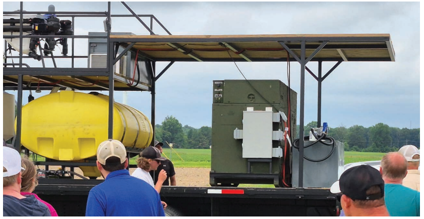
A diesel-powered generator costs significantly more than gas-driven units but is more durable and dependable under field conditions. Their heavier weight makes them less portable.
