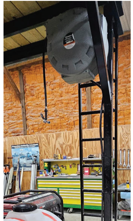
Hose reels for hoses delivering clean water.
