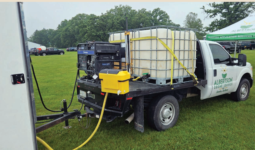
Due to the trailer's space and weight limitations, the two tanks of clean water and the electric generator are carried on the truck bed. The yellow tank holds clean water to wash hands and clean the drone after the application is completed.
