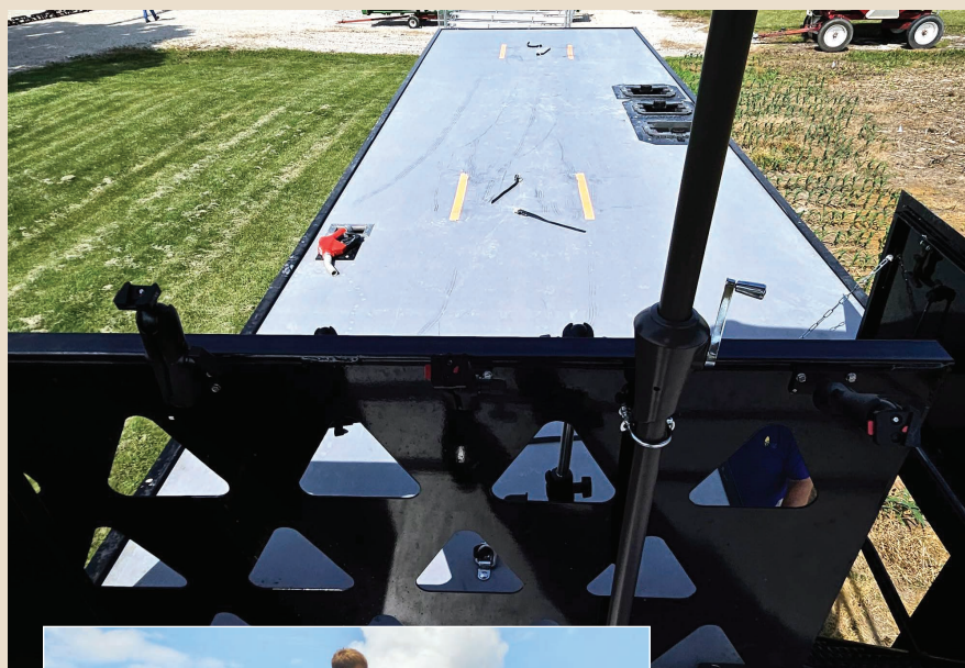
Top view of the trailer's platform. There is enough space on the platform for two drones to land. This also shows that the filling nozzle and charging stations protrude onto the upper deck so the whole operation can be conducted from there without constantly going from the top deck to the lower deck.
