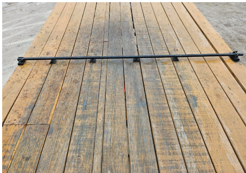
Chemical spills can soak into wood decks, and these decks can also become slippery when wet. Adding a coating to keep chemicals from soaking into the wood and adding nonslip surfaces are best practices when building your truck/trailer setup.
