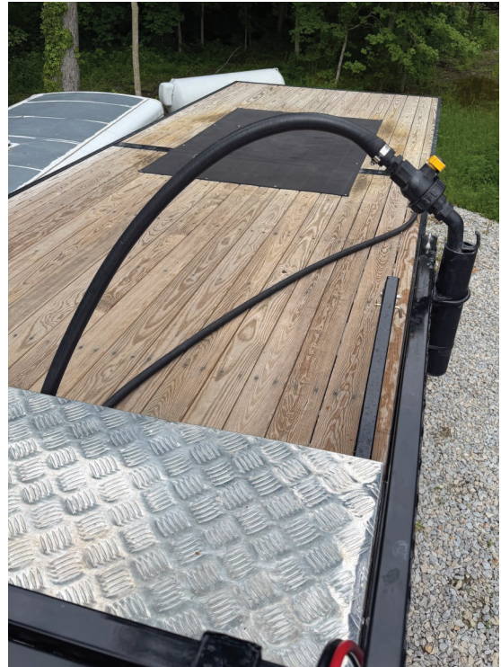
The nozzle used to fill the sprayer has a sleeve that it can be placed into. This will help to prevent a lot of bending during the day.
