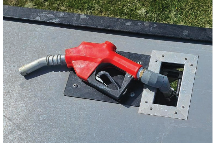
A gasoline-type nozzle that is used to fill a drone. The drone in this operation has a modified gas cap that the nozzle will fit into.
