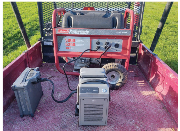
While it is not common, a generator may list two numbers to describe the power produced. This Coleman generator highlights two different numbers related to wattage—6,250 and 5,000. The first is the peak output, while the second is the constant running power. Make the best purchase when comparing generators by using the constant running power.
