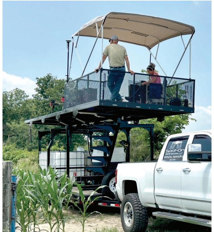
An open canopy, providing shade for the entire operator's station and batteries.
