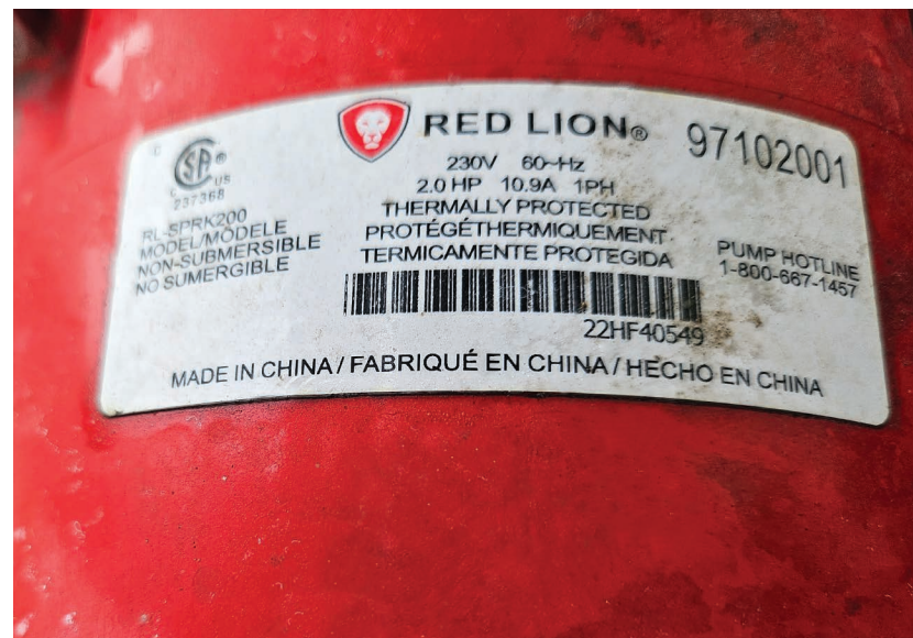
This model of a Red Lion pump can deliver 76 gallons per minute and could take care of the needs of most drone trailers.
