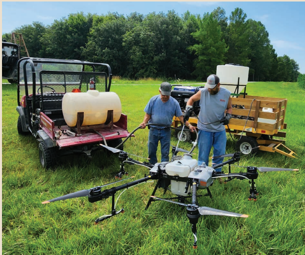
Filling the drone from an auxiliary tank with a premixed pesticide, which is placed on an all-terrain vehicle.
