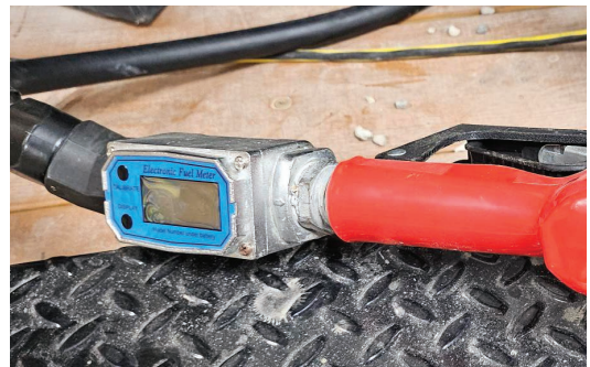
Flowmeters in operation on drone trailers.
