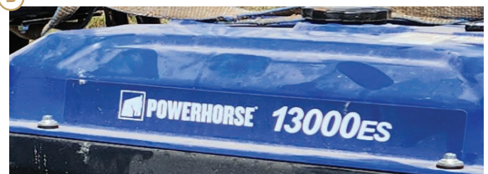
(A) This Westinghouse generator lists 28,000 watts (28 kilowatts) of peak power. Its constant running power is listed as 20 kilowatts in the product's brochure. (B) This generator lists 13,000 watts (13 kilowatts) of peak power. Its constant running power is rated at 10.5 kilowatts if it runs on gasoline.
