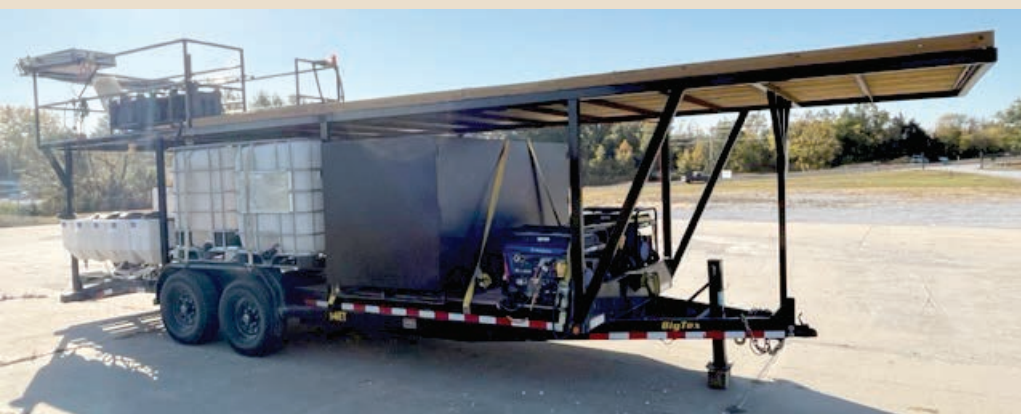
A series of small white totes are part of an auto-mixer. Each tote can contain a specific pesticide that can be metered into the water line running to the application drone.
