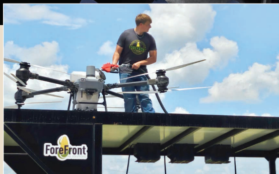
Top view of the trailer's platform. There is enough space on the platform for two drones to land. This also shows that the filling nozzle and charging stations protrude onto the upper deck so the whole operation can be conducted from there without constantly going from the top deck to the lower deck.
