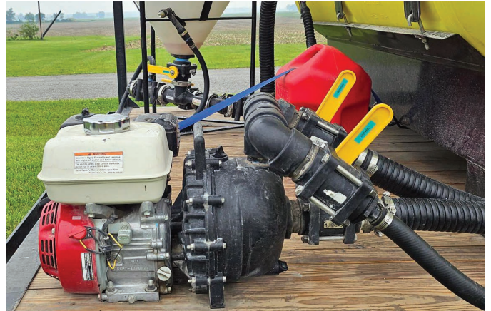
Here a gas Honda engine and Banjo pump form a single unit.
