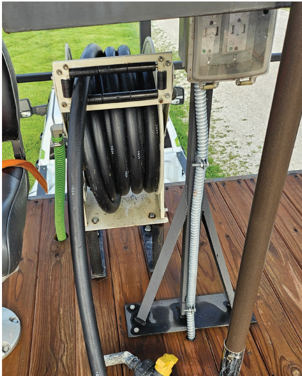
The hose reel has to be matched to the size of the hoses being used to fill the drone.
