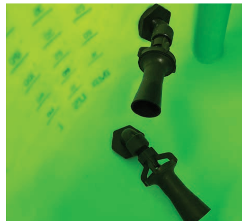
The inside of a tank with two eductors to provide current to suspend or resuspend pesticides.
