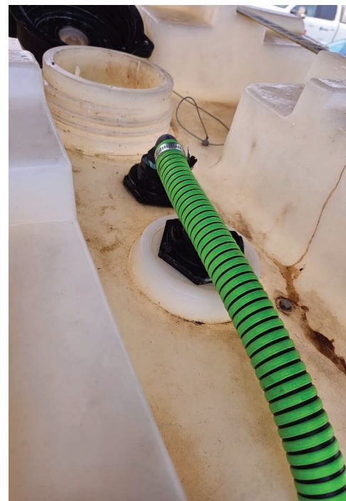
A hose running to the top of the tank to allow for recirculation of the fluid.
