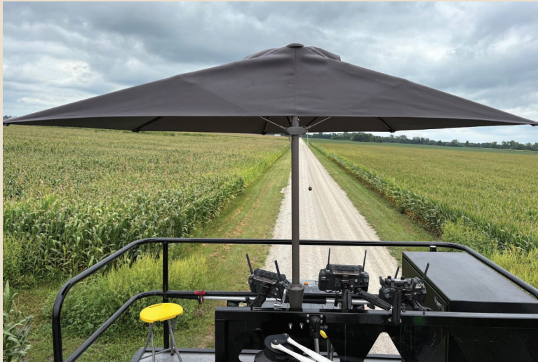
The work area showing the placement of the controllers and the umbrella. Notice that the umbrella does not have flaps coming down, allowing the drone pilot to clearly see the platform and the drone as it flies over the fields.
