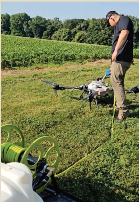
A pesticide can be added directly to the spray tank or to the 60-gallon inductor tank when larger batches are required. A 12-volt electric pump is used to move the water.
