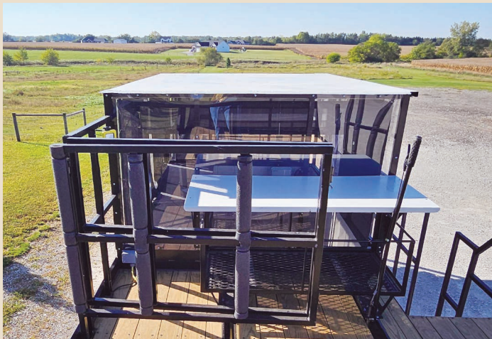
The cart is equipped with battery chargers. When charging, they are under a table, which provides shade to keep the batteries cooler.
