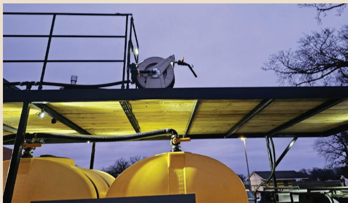
Each side has its own hose reel to fill the drones. Hose reels can reduce clutter and make cleanup and teardown fast, necessary for a drone business.
