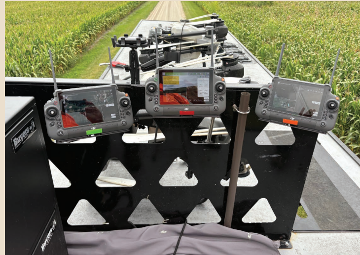
The work area showing the placement of the controllers and the umbrella. Notice that the umbrella does not have flaps coming down, allowing the drone pilot to clearly see the platform and the drone as it flies over the fields.
