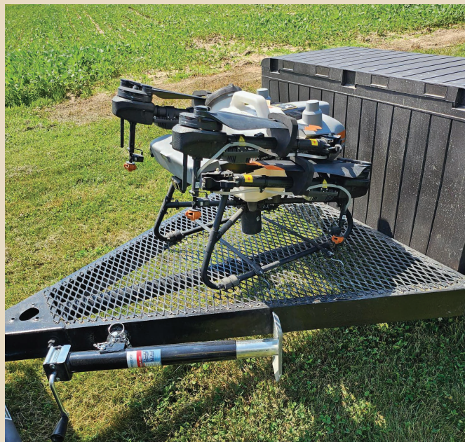
A small spray drone fits well on the front end of the trailer, where it is secured when transported.
