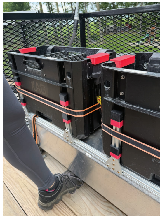
A battery box is elevated to allow this person to get their feet underneath. That allows the operator to lift the batteries straight up using the form that is used by weightlifters. This will help reduce fatigue and back pain. The actual height of the battery box will depend on the height of the individuals handling the drone batteries.
