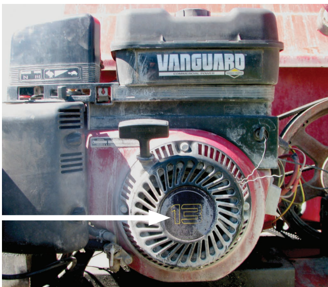
This Vanguard engine has a gross horsepower rating of 13, as marked on the front of the engine.
