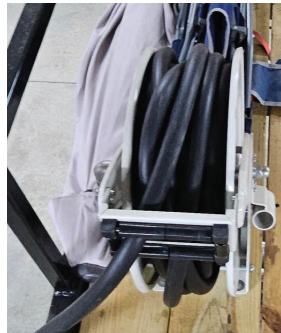
Hose reels for hoses delivering clean water.
