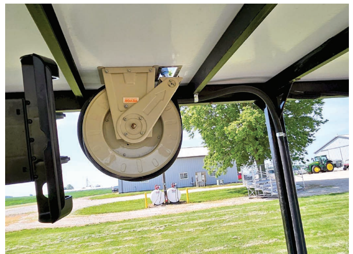
Make sure your hose reel's diameter is large enough that the hose does not kink when rolled up. Kinking may reduce flow rate and may not be an easy problem to identify when trying to diagnose the cause of a slow refill.
