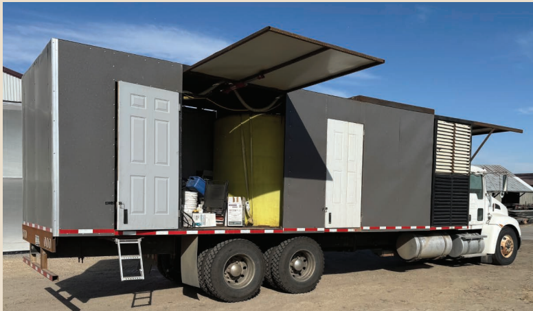
An enclosed trailer built by the drone operator. The trailer has a powerful 125-kilowatt Cummins Onan diesel generator (1) and an enclosed lift (2).
