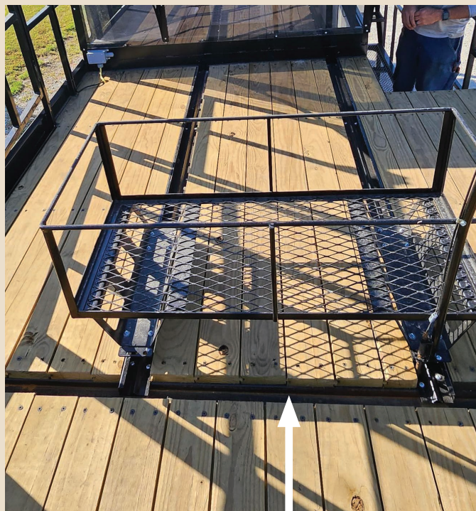
The cart rolls out to the drone with the charged battery. This allows the depleted battery to go directly into the charger, speeding up the operation by 20 seconds. More important, the technician doesn't have to bend, reducing fatigue. A key advantage to this operation is there is no reason to go out to the end of the platform since swapping the battery and refilling the drone is done in the center. The dark gap between the wooden sections (white arrow) allows spills on the platform to drain to the sides to the trailer.
