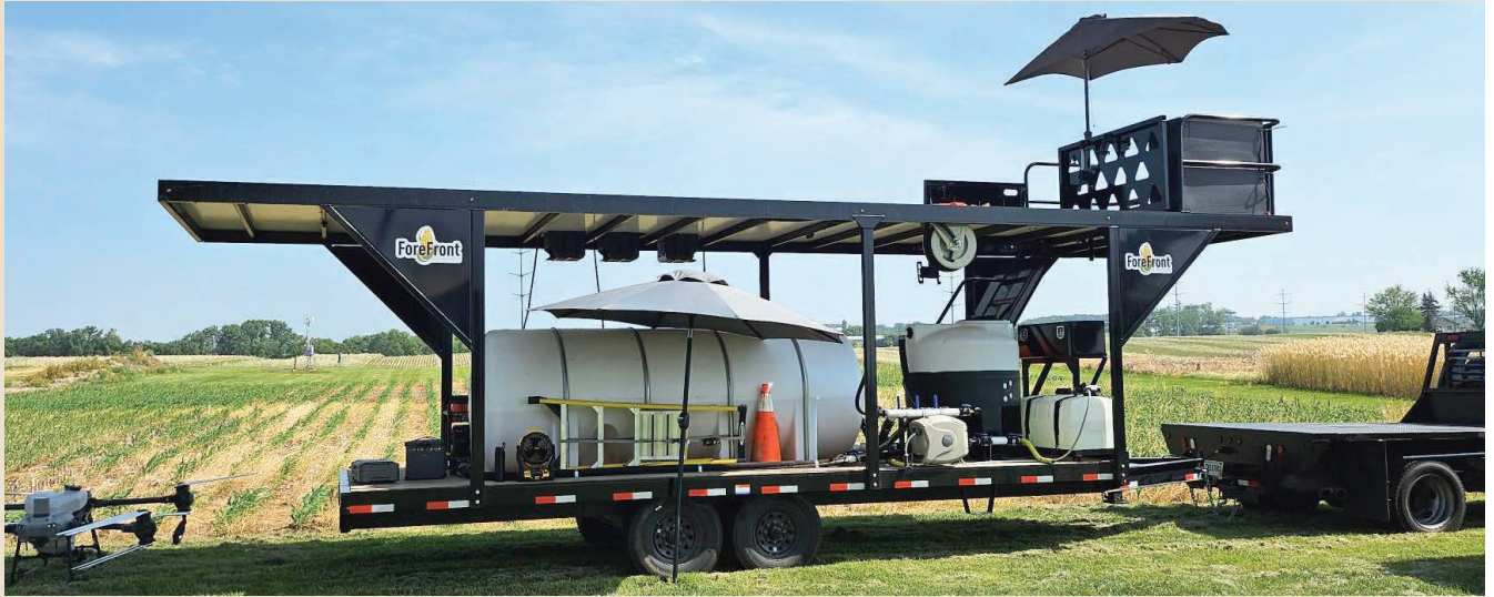
A wide-angle view of a very efficient drone trailer. The pilot works within the area protected by railings to avoid falling off and to protect them from the drone just in case a drone malfunctions.
