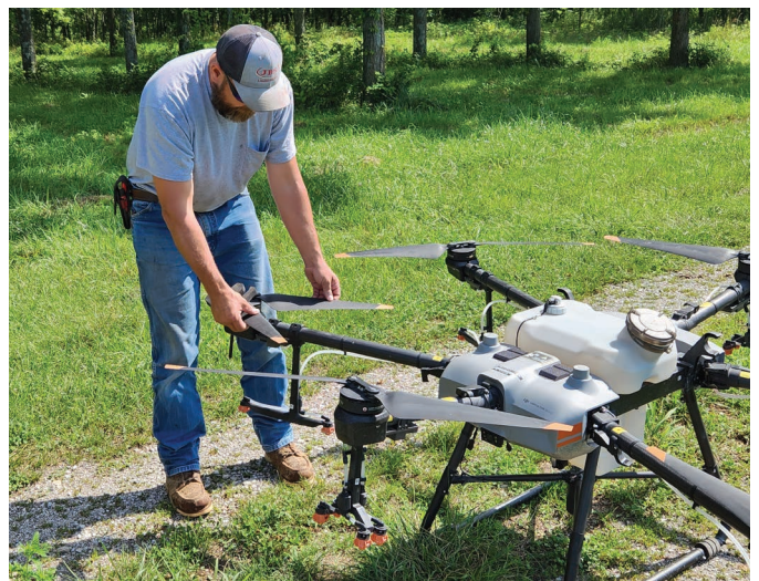
Make sure the power is shut down when inspecting blades.
