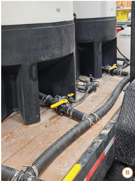
(A) A clear PVC-based suction hose showing the ribs that prevent the hose from collapsing. (B, C, D) Suction hoses in use on drone trailers.
