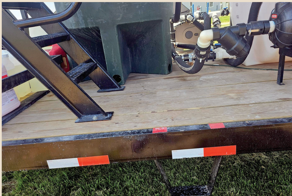
Red tape on the edge of the trailer deck marks the location of the steps for stepping down onto the ground.
