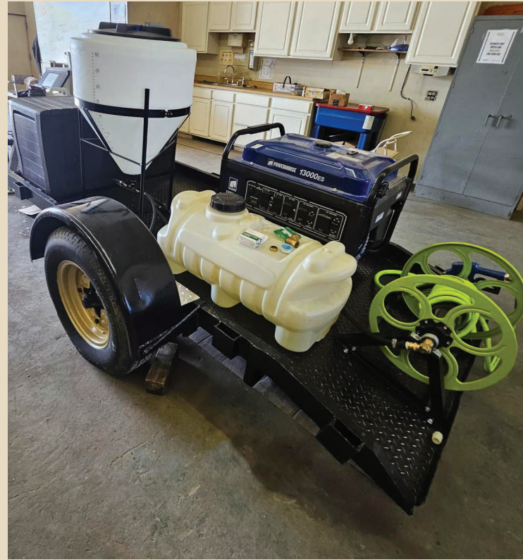
A limited-use trailer outfitted with an electric generator, a cone inductor tank for mixing, a storage box, a water tank, and a hose reel.
