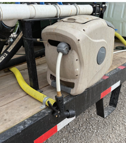
Make sure your hose reel's diameter is large enough that the hose does not kink when rolled up. Kinking may reduce flow rate and may not be an easy problem to identify when trying to diagnose the cause of a slow refill.
