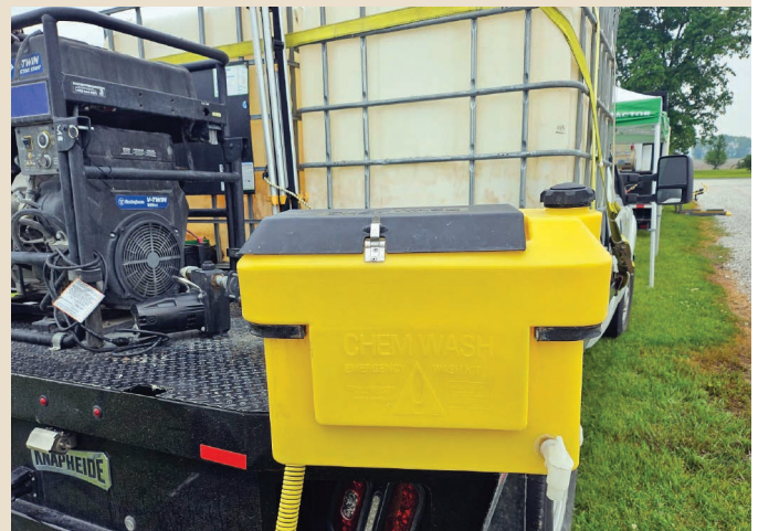
Due to the trailer's space and weight limitations, the two tanks of clean water and the electric generator are carried on the truck bed. The yellow tank holds clean water to wash hands and clean the drone after the application is completed.
