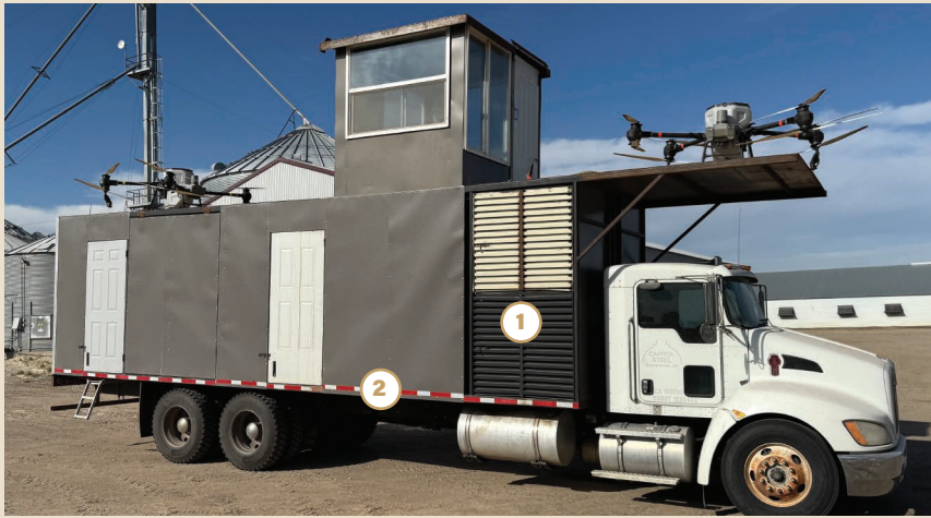
An enclosed trailer built by the drone operator. The trailer has a powerful 125-kilowatt Cummins Onan diesel generator (1) and an enclosed lift (2).
