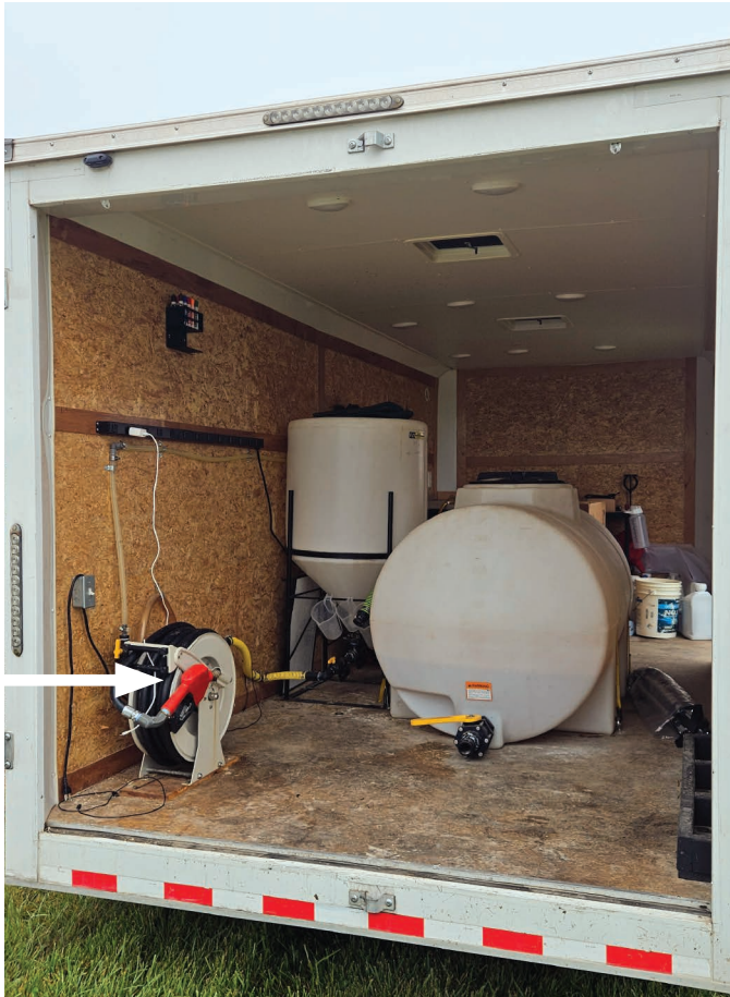
A gasoline-type nozzle that is used to fill a drone. The drone in this operation has a modified gas cap that the nozzle will fit into.
