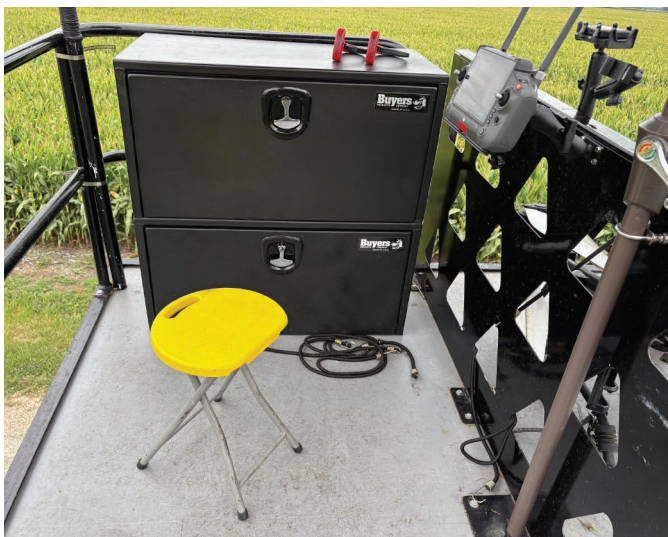
Proper mounting for a controller not in positive hand control. There is a convenient hook for the controller while the pilot fills up the drone or swaps batteries.
