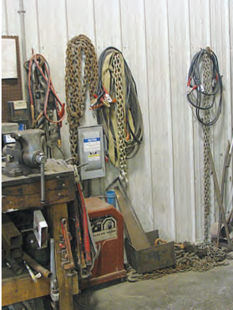
These are nice chains stored indoors, but it isn't clear what their ratings are or what they should be used for. It would be wise to permanently attach labels with their ratings to each chain.
