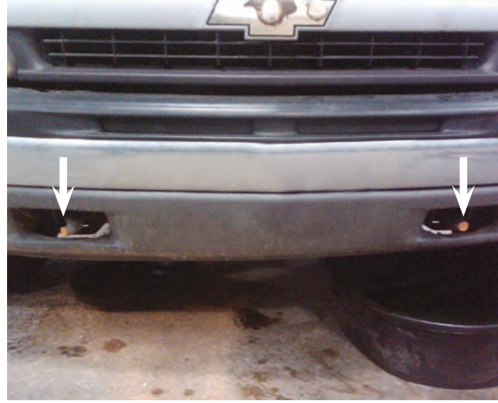
These tow hooks were ripped off the truck when the operator attempted to extract the truck and a nurse tank trailer at the same time. The operator should have unhooked the trailer and pulled the truck out first, and then extracted the trailer.
