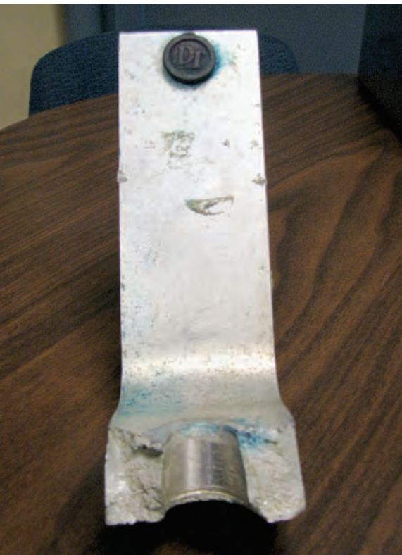
An attempt was made to pull out a sprayer with the hitch. The force exceeded the ball, shank, and insert, which caused the metal to recoil into the equipment.
