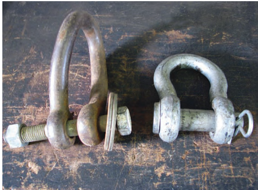
Never replace the original pin that came with your device with bolts from your bins or local hardware stores (left). If you need to replace the pin, replace it with a pin that is comparable to the pin that came with the original equipment at the time of purchase.
