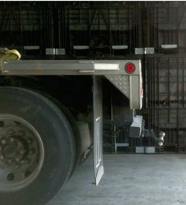
The insert and ball has been bent downward from the forces being applied on it from pulling out a stuck vehicle. A little more force could have easily broken the ball or insert.
