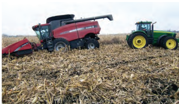
When attempting to extract equipment, the only people who should be seen are the drivers.
