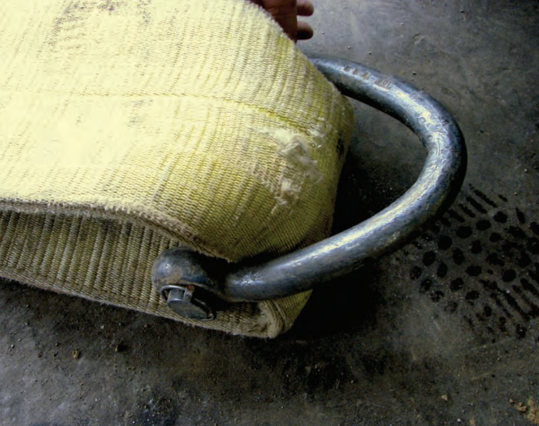
When possible, attach the strap or rope so that it is on the pin and not on the body of the clevises.
