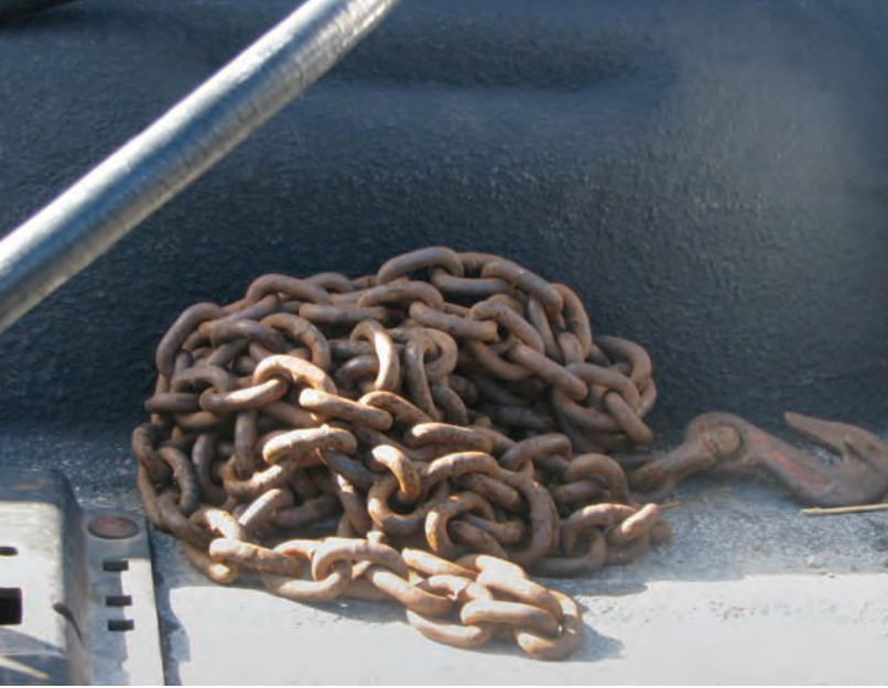
These chains are ready for use and have been field-tested in years past. The problem is that a single chain with an unknown grade cannot pull everything. The chain will fail when it finally meets its match.
