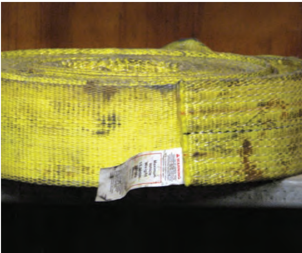
Keep this recovery strap in a container to protect it against damage from grease and sunlight.
