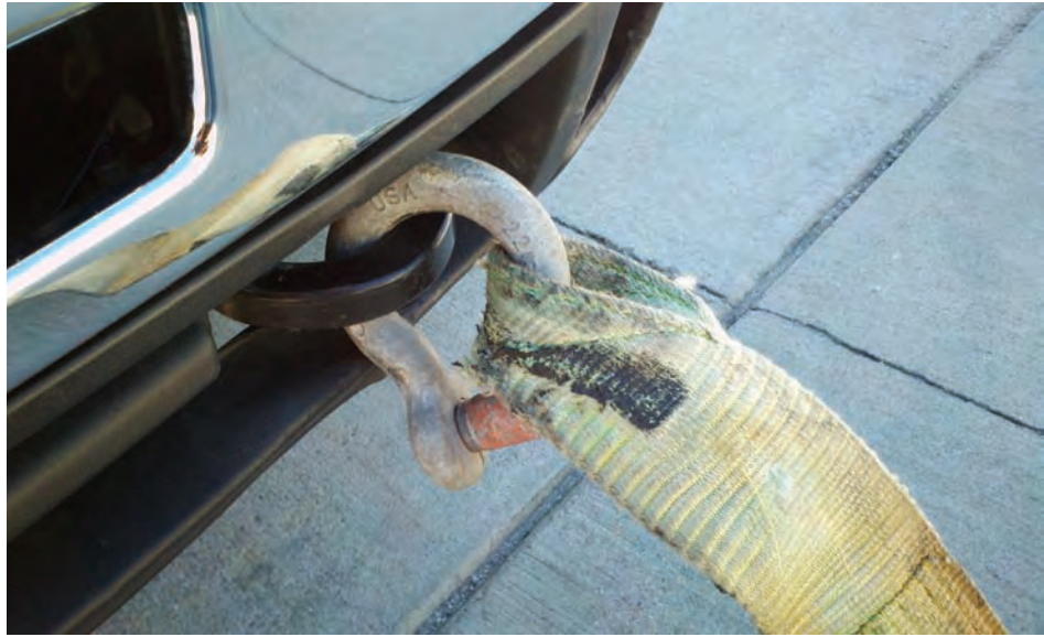
An improper strap attachment can pull apart the clevis.
