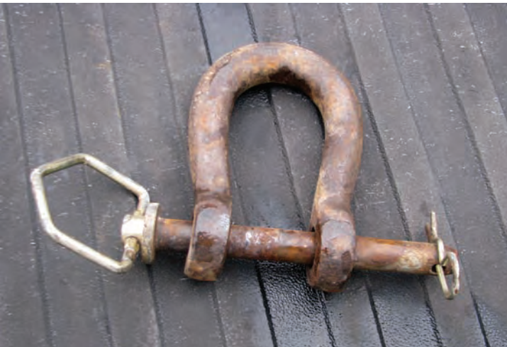
Using a regular hitch pin in lieu of what came with the clevis is a mistake.
