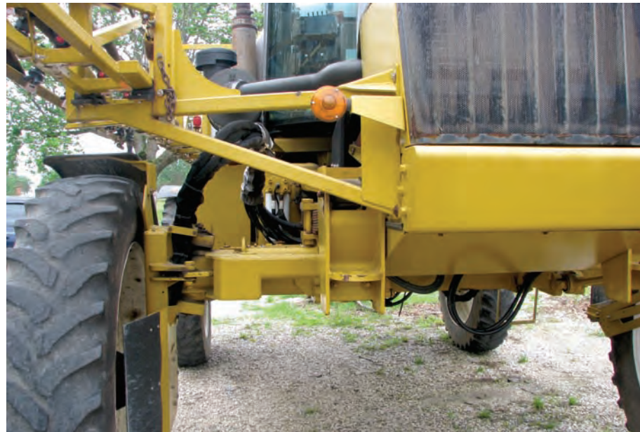
These tow hooks were ripped off the truck when the operator attempted to extract the truck and a nurse tank trailer at the same time. The operator should have unhooked the trailer and pulled the truck out first, and then extracted the trailer.
