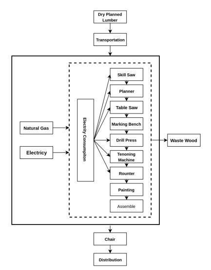
Figure 2: Production LCI system boundary. The dash line area are the main production process and bold black line area is the system boundary
