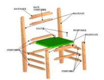
Figure 1: Exploded view of 14" chair components
