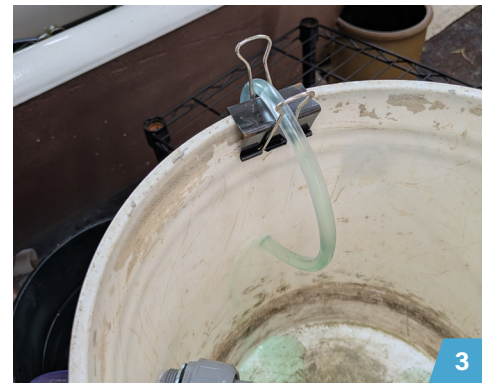
3 Start the pump and watch water flow into the upper bucket
