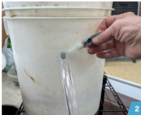
2 Add glue around the hole to prevent leaking
