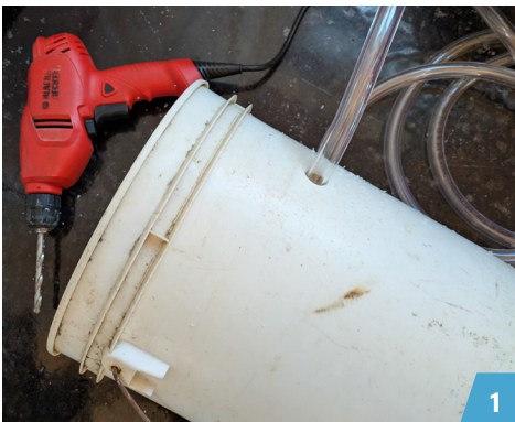
1 Drill a hole and push the tubing through
