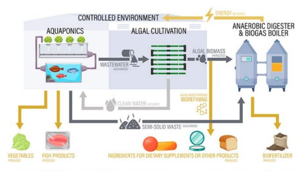
Our integrated aquaponics system will include the traditional components of an aquaponics system along with the additional algal cultivation unit, biogas boiler and anaerobic digester.
