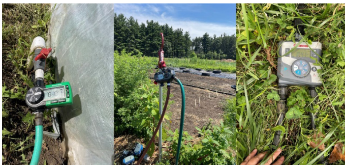
Figure 20. Different types of timers are used to control automatic irrigation systems on small farms.
