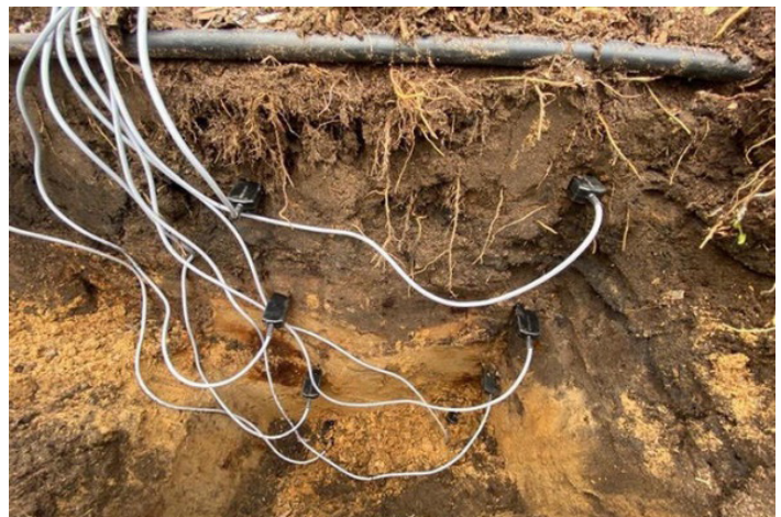
Figure 23. Sensors measuring volumetric water content were placed at different soil depths. The photo was adapted from Dong, Y. (2023). "Irrigation Scheduling Methods: Overview and Recent Advances."
