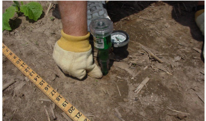
Figure 22. Installing a tensiometer in the soil.
