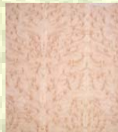
Figure 1. Birdseye in maple. Rotary cut, three-piece book match (origin: North America). Logs with high density patterns like this that are consistent and clean will demand a premium price [4] .
