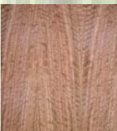
Figure 3. Beeeswing in eucalyptus. Quarter cut, three-piece book match (origin: Australia, Europe, and North America). Also called Tasmanian oak. Highly figured logs are highly prized.
