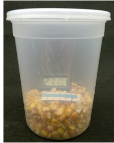
Figure 1. Prototype moisturemeter that uses humidity/temperature devices
