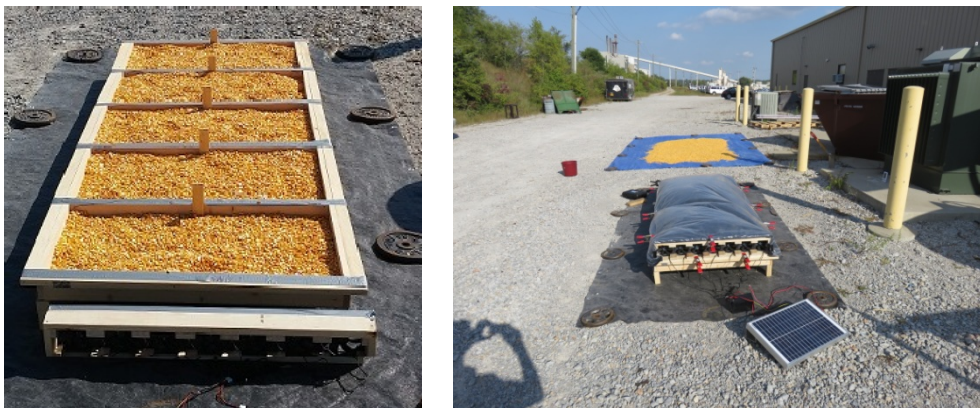
Figure 7. POD with shelled maize in its trays (left) prior to addition of the plastic covering and (right) POD covered with plastic along with shelled maize drying on the tarp (rear). In the picture on the left, the seven fans enclosed in a frame can be seen on the tarp in front of the first POD tray.
