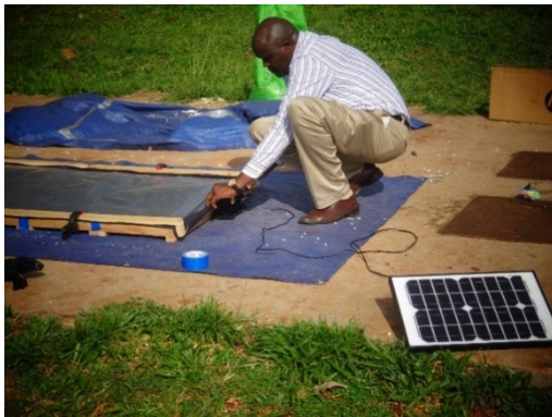
Figure 4. Preparation for the drying test comparing performance of the POD dryer with that of an open tarp. Tests were conducted by Mr. Patrick Ketiemi and his assistants at KALRO in Kenya
