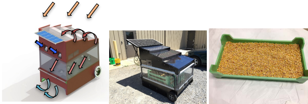
Figure 14. The multipurpose solar dryer, left to right: engineering rendering (left), assembled unit (center) and drying tray (right).
