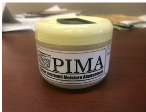
Figure 1. Standardized product of hygrometer embedded in a plastic jar.
