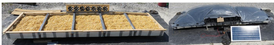
Figure 4. Picosolar crOp Dryer (POD) with aluminum fan frame tested during the summer of 2018. Left picture shows the maize in the trays with the fan frame positioned along the side of the trays. The right picture shows the POD trays with the plastic sheet in place, fans running, and a 30 Watt solar panel.
