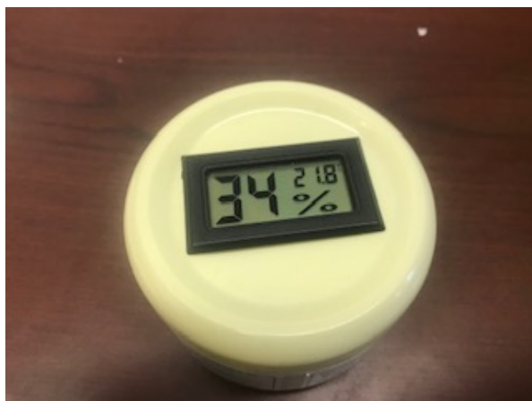
Figure 1. Standardized product of hygrometer embedded in a plastic jar.
