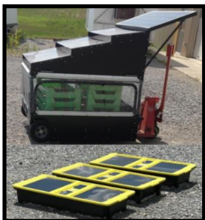
Figure 3. Multipurpose cabinet solar dryer and drying trays
