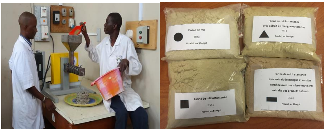
Figure 7. Single-screw extruder being used to produce instant extruded weaning foods enriched with select fruits and or vegetables, or with commercial micronutrients.
