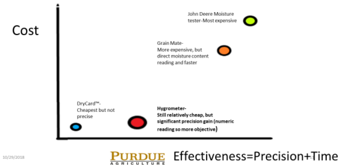
Figure 4. Comparison of hygrometer to other moisture meters on market
