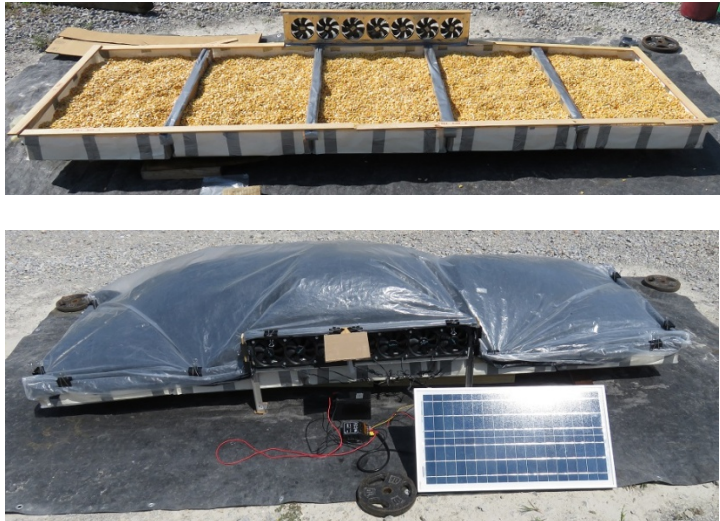
Figure 5. Picosolar crOp Dryer (POD) with aluminum fan frame tested during the summer of 2018. Upper picture shows the maize in the trays with the fan frame positioned along the side of the trays. The lower picture shows the POD trays with the plastic sheet in place fans running, and a 30 Watt solar panel.
