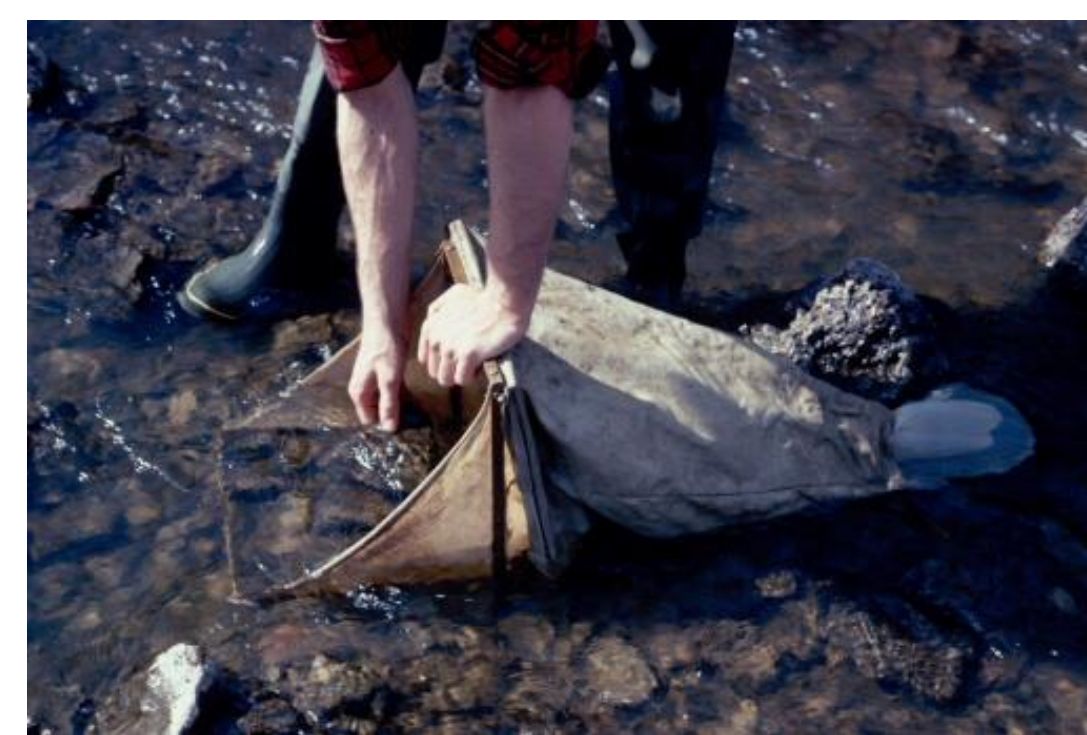
Figure 3. Surber sampler for macroinvertebrates (ASLO – aslo.net)
