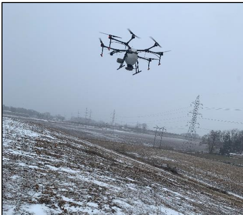
The drone in action spreading seed on the hillside of the mound.
