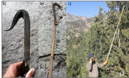
**Figure 3.** Chilgoza pine cone removal hook, b) hook attached to pole and, c) cone collection with hook.
