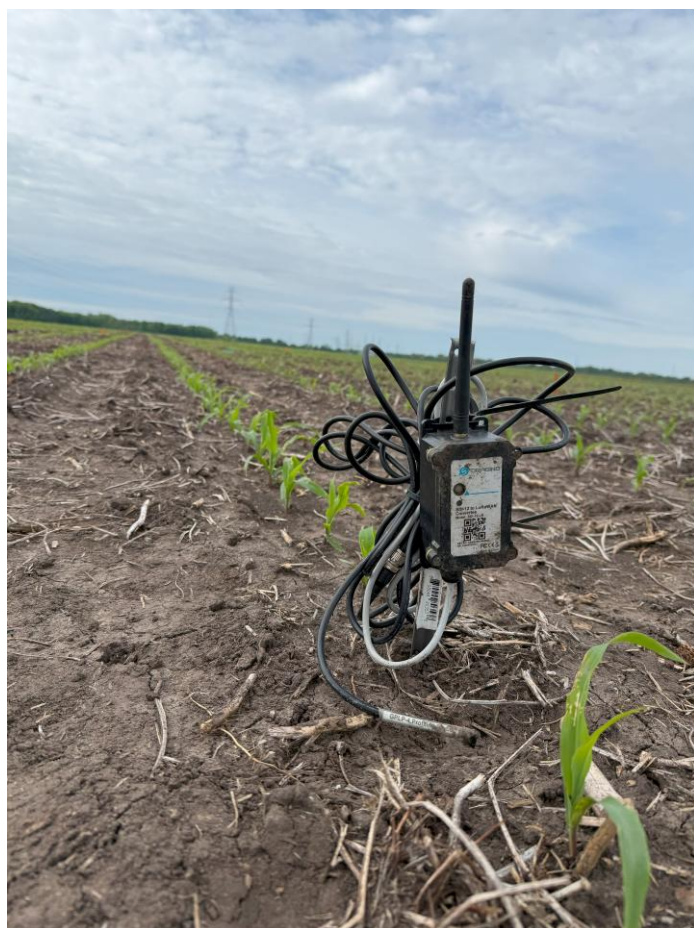
Figure 3. Hydrology sensor on the IoT4Ag research trial at ACRE, West Lafayette, IN. Photo taken on May 27 th .
