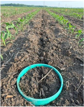
**Figure 2.** Collar for N2O measurements installed at the Corteva's trial after sidedress application at ACRE, West Lafayette, IN.
