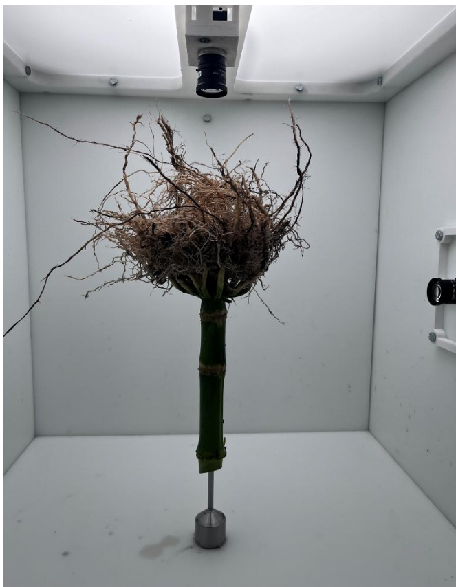
Figure 1. Scanning root at R2 growth stage using the imaging box at Beck's Hybrids facility center.
