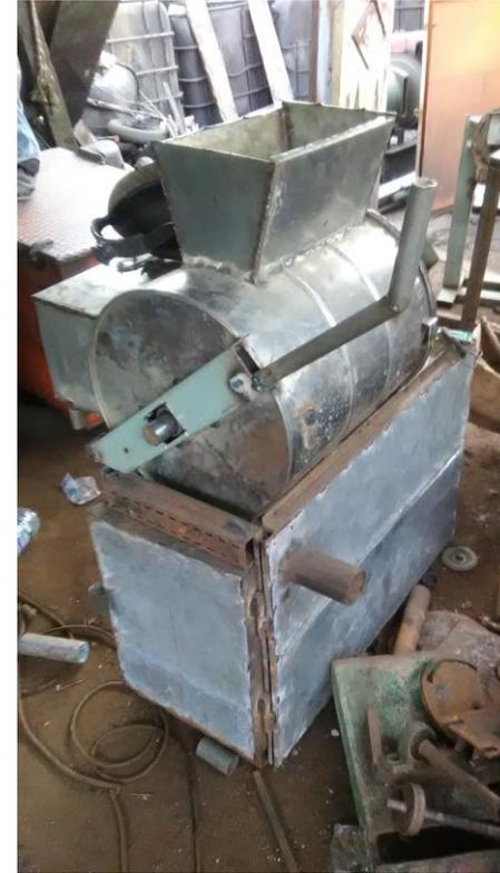
The Integrated Mobile Cassava Peel Processing Machine developed by us processes fresh cassava peels, through particle size reduction, in three distinct stages that include: (1) Grinding (2) Dewatering (3) Drying. This drastically reduces cyanogenic glycosides with improved shelf life of up to six months.
