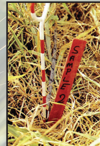
12. The sample number should be written on the anchor stake at the beginning of the buffer zone.
